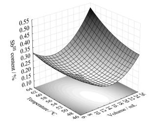
Figure 2. Response surface for the %Sb<sup>III</sup> property out of total Sb in MA compounds obtained via SbCl<sub>5</sub> synthetic route.
