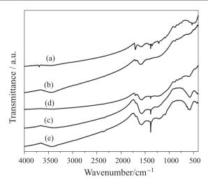
**Figure 1.** Infrared spectra for the (a) AC sample (activated carbon), and for the (b) 2.5IAC, (c) 5IAC, (d) 10IAC and (e) 15IAC samples (activated carbon-supported iron oxide). The numbers represent the iron amount (wt.%) in the solids.
