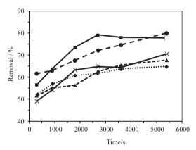
**Figure 8.** Methylene blue removal by adsorption on the catalysts as a function of time during the Fenton reaction, AC sample ( $\times$ ) (activated carbon), and 2.51AC ( $\blacklozenge$ ), 51AC ( $\bigstar$ ), 101AC ( $\blacklozenge$ ) and 151AC ( $\blacksquare$ ) samples (activated carbon-supported iron oxide). The numbers represent the iron amount (wt.%) in the solids.
