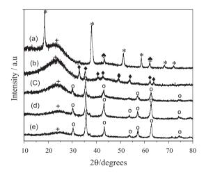
**Figure 2.** X-ray diffratograms for the (a) AC sample (activated carbon), and for the (b) 2.51AC, (c) 51AC (d) 10IAC and (e) 15IAC samples (activated carbon-supported iron oxide). The numbers represent the iron amount (wt.%) in the solids. ( $\bigstar$ ): magnesium oxide (MgO); (\*) magnesium carbide (Mg<sub>2</sub>C<sub>3</sub>); (+) activated carbon; (0) magnetite (Fe<sub>3</sub>O<sub>4</sub>); ( $\bigstar$ ) hematite (Fe<sub>2</sub>O<sub>3</sub>).
