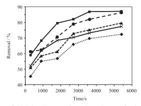
**Figure 7.** Methylene blue removal over the catalysts as a function of time during the Fenton reaction: AC sample ( $\times$ ) (activated carbon), and 2.5IAC ( $\blacklozenge$ ), 5IAC ( $\bigstar$ ) 10IAC ( $\blacklozenge$ ) and 15IAC ( $\blacksquare$ ) samples (activated carbon-supported iron oxide). The numbers represent the iron amount (wt.%) in the solids.
