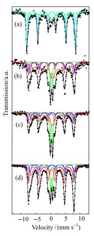
**Figure 3.** Mössbauer spectra for the (a) 2.5 IAC, (b) 5IAC, (c) 10IAC and (d) 15IAC samples (activated carbon-supported iron oxide). The numbers represent the iron amount (wt.%) in the solids. The blues lines represent magnetically blocked magnetite or hematite, the red one the relaxing magnetite or hematite and the green ones represent supermagnetic hematite.
