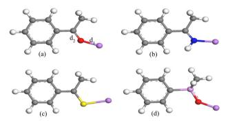
**Figure 2.** Optimized structures of the Li<sup>+</sup> complexes with the hydrogen atom as the *para*-substituted group. The d<sub>1</sub> (bond length between the lithium cation and the O, N or S atom) and d<sub>2</sub> (C=O, C=N, C=S and P=O double bond) distances for the (a) carbonyl, (b) imino, (c) thiocarbonyl, (d) phosphoryl compounds are shown. The lithium cation is shown in pink color. See online version for color visualization.
