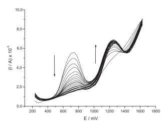
**Figure 2.** Differential pulse voltammograms of the mixture of *cis*-[RuCl<sub>2</sub>(P-P)(Cl-bipy)] with pyridine in CH<sub>2</sub>Cl<sub>2</sub>. Experimental conditions: 0.1 mol L<sup>-1</sup> tbap, 20 °C, 1/10 complex/ligand, Pt *vs*. Ag/AgCl. Sweep rate: 170 mV s<sup>-1</sup>.
