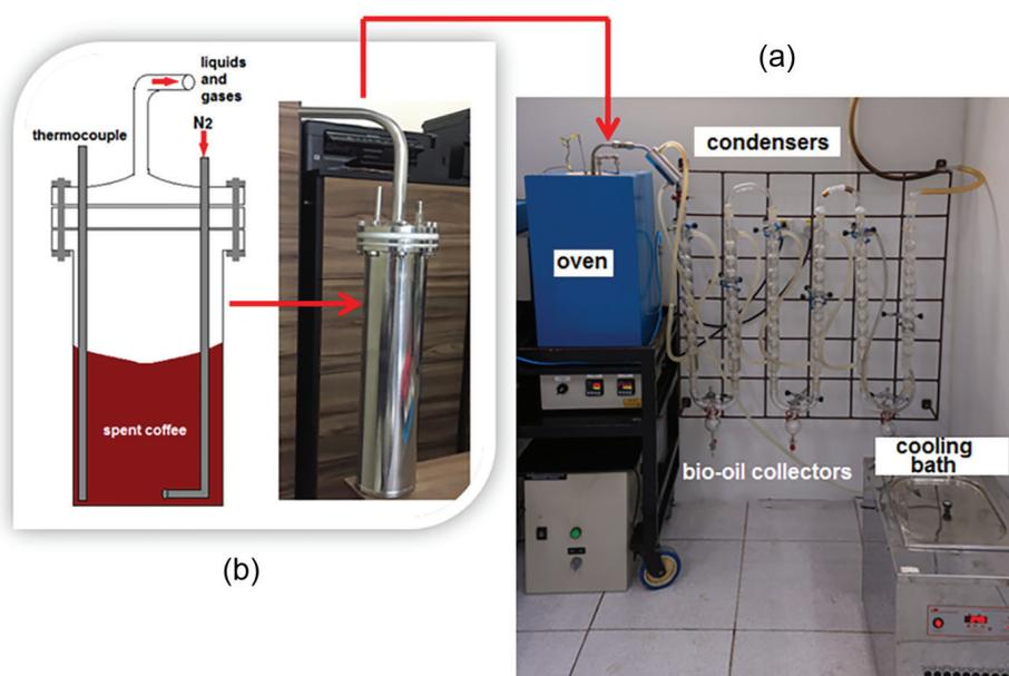
**Figure 1.** Illustration of the pyrolytic system: (a) Photograph of the whole system (oven, condensers and cooling bath); (b) details of the stainless-steel reactor.
