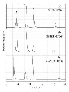
**Figure 7.** Chromatograms showing the separation of a test mixture with stationary phases prepared by thermal immobilization (110 °C) of PMTDS on (a) silica, (b) titanized silica and (c) zirconized silica particles. Chromatographic conditions: mobile phase: methanol:water (70:30 v/v), flow rate: 0.3 mL min<sup>-1</sup>; UV detection: 254 nm; injection volume: 5 µL. Peak identifications: 1- uracil, 2- phenol, 3- N,N-dimethylaniline, 4- naphthalene and 5- acenaphthene.
