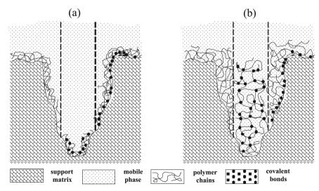
Figure 3. Types of polymeric deposition on a chromatographic support. (a) Coating of the pore walls or (b) filling of the pore volume. Adapted from Reference 53.
