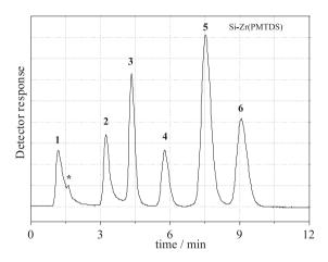
**Figure 8.** Chromatogram showing the separation of a pesticide mixture with a Si-Zr(PMTDS) phase. Chromatographic conditions: mobile phase: methanol:water (50:50, v/v), flow rate: 0.3 mL min<sup>-1</sup>; UV detection: 235 nm; injection volume: 5  $\mu$ L. Peak identifications: 1- imazethapyr, 2- cyanazine, 3- carboxin, 4- atrazine, 5- diuron, 6- linuron and \*- sub-product from imazethapyr. Adapted from Ref. 93.
