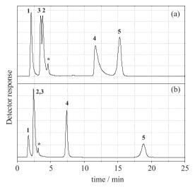
**Figure 5.** Chromatograms showing the separation of a test mixture with Si-Zr(PMTDS) phases: (a) not end-capped and (b) end-capped. Chromatographic conditions: mobile phase: methanol:water (55:45 v/v), flow rate: 0.3 mL min<sup>-1</sup>; UV detection: 254 nm; injection volume: 5 µL. Peak identifications: 1- uracil, 2- aniline, 3- phenol, 4- N,N-dimethylaniline and 5- naphthalene.
