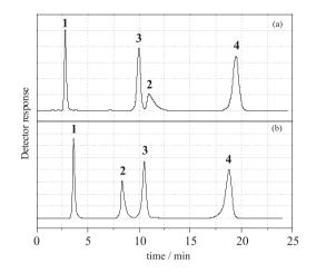
**Figure 4.** Chromatograms showing the separation of a test mixture with a thermally immobilized (120 °C) titanized-silica-based PMOS stationary phase using (a) 8 h and (b) 24 h. Chromatographic conditions: mobile phase: methanol:water (70:30 v/v), flow rate: 0.3 mL min<sup>-1</sup>; UV detection: 254 nm; injection volume: 10  $\mu$ L. Peak identifications: 1- phenol, 2- N,N-dimethylaniline, 3- naphthalene, 4-acenaphthene. Adapted from Ref. 95.
