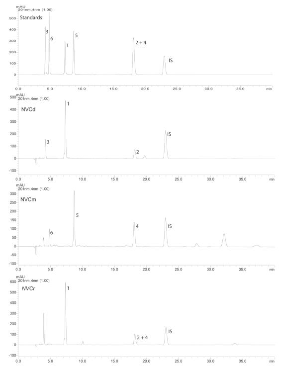
Figure 2. RP-HPLC chromatograms of NVCd, NVCr, NVCm and IS (manool) in comparison with the respective standards. (1) (–)-polyalthic acid; (2) (13E)-ent-labda-7,13-dien-15-oic acid; (3) ent-8(17)-labden-15,18-dioic acid; (4) (–)-copalic acid; (5) (–)-3 $\beta$ -acetoxycopalic acid and (6) (–)-3 $\beta$ -hydroxycopalic acid.
