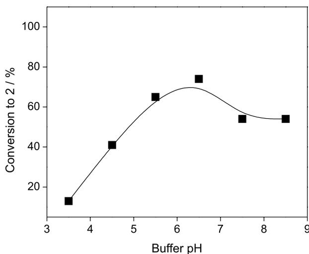
**Figure 4.** Effect of buffer pH on the bioreduction of **1** catalyzed by baker's yeast in water/*n*-hexane biphasic system with addition of DMSO. Reaction conditions: BY (4 g), **1** (140 mg), 30 mL of citrate/phosphate/borate buffer (0.1 mol L<sup>-1</sup>, pH 3.5-8.5), 28.5 mL *n*-hexane, 1.5 mL DMSO (2.5% v/v), 35 °C, 5 h, magnetic stirring.
