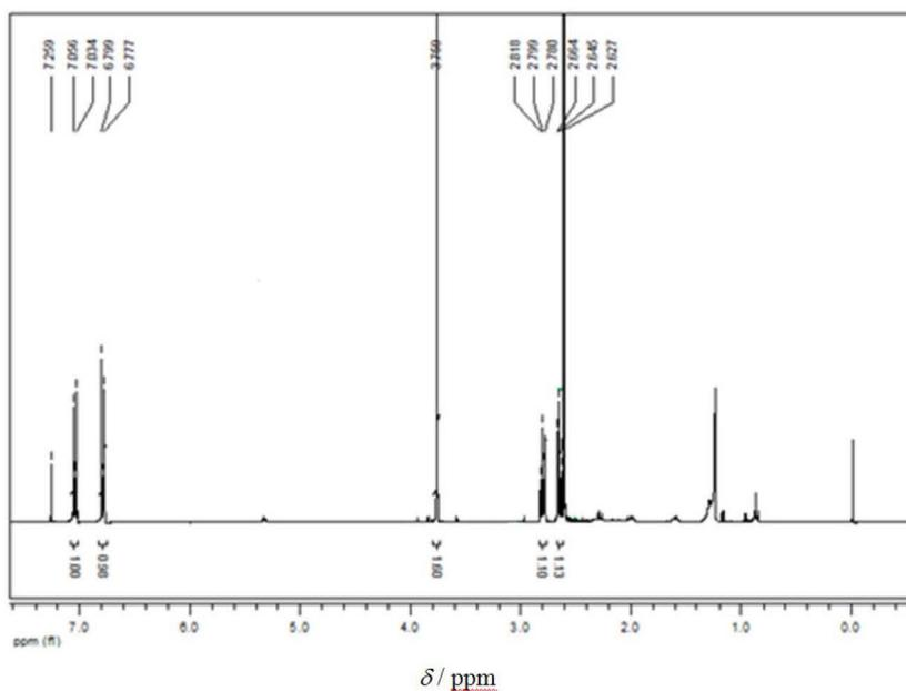
**Figure S3.**  $^1\text{H}$  NMR spectrum ( $\text{CDCl}_3$ , 400 MHz) of 1,5-bis(4-methoxyphenyl)-3-pentanone.
