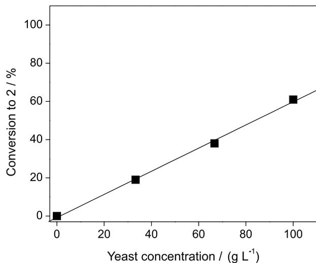
**Figure 1.** Effect of the yeast concentration on the bioreduction of **1** catalyzed by baker's yeast in water/*n*-hexane biphasic system with addition of DMSO. Reaction conditions: BY (0-6 g), **1** (290 mg), 30 mL of citrate/phosphate/borate buffer (0.1 mol L<sup>-1</sup>, pH 5.5), 28.5 mL *n*-hexane, 1.5 mL DMSO (2.5% v/v), 35 °C, 5 h, magnetic stirring.
