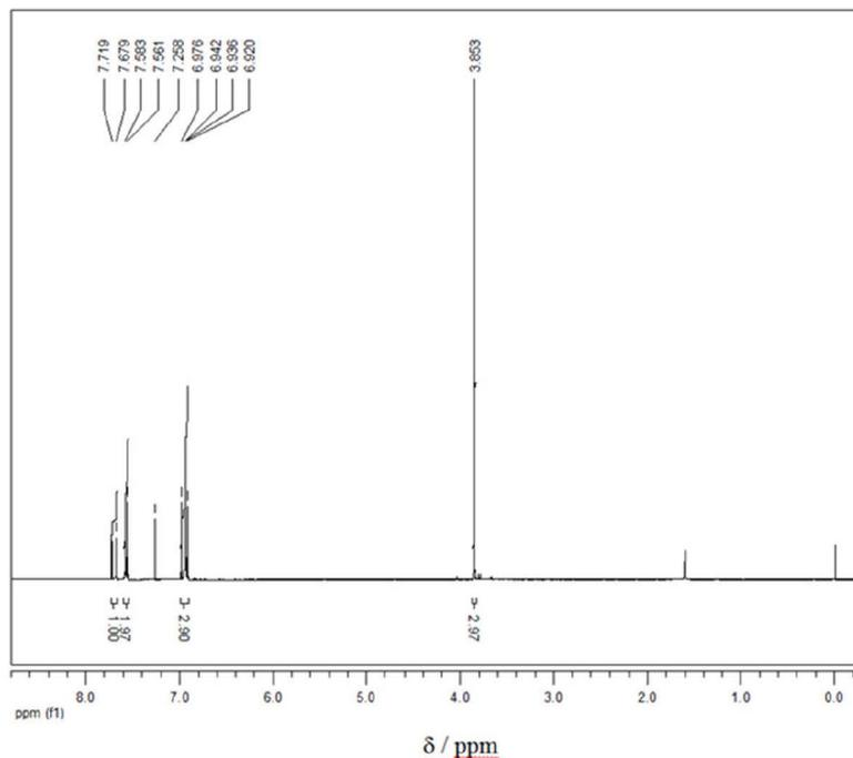
**Figure S2.**  $^1\text{H}$  NMR spectrum ( $\text{CDCl}_3$ , 400 MHz) of (1*E*,4*E*)-1,5-bis(4-methoxyphenyl)-1,4-pentadien-3-one.
