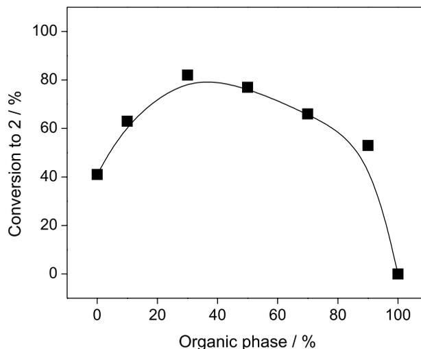
**Figure 5.** Effect of  $V_{aq}/V_{org}$  on the bioreduction of **1** catalyzed by baker's yeast in water/*n*-hexane biphasic system with addition of DMSO. Reaction conditions: BY (4 g), **1** (140 mg), 0.0-58.5 mL of citrate/phosphate/borate buffer (0.1 mol L<sup>-1</sup>, pH 6.5), 0.0-58.5 mL *n*-hexane, 1.5 mL DMSO (2.5% v/v), 35 °C, 5 h, magnetic stirring.
