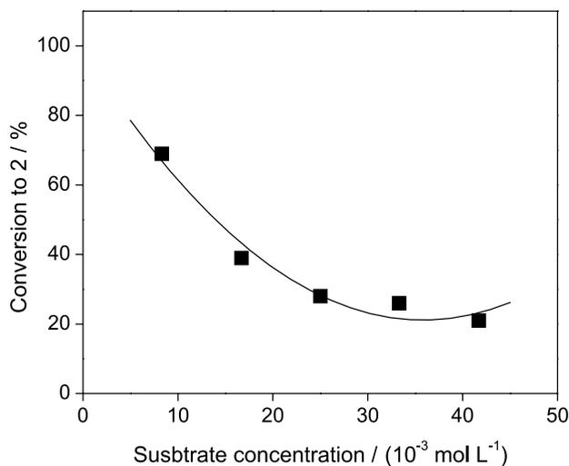
**Figure 2.** Effect of the substrate concentration on the bioreduction of **1** catalyzed by baker's yeast in water/*n*-hexane biphasic system with addition of DMSO. Reaction conditions: BY (4 g), **1** (140-720 mg), 30 mL of citrate/phosphate/borate buffer (0.1 mol L<sup>-1</sup>, pH 5.5), 28.5 mL *n*-hexane, 1.5 mL DMSO (2.5% v/v), 35 °C, 5 h, magnetic stirring.
