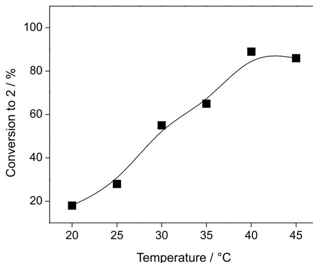
**Figure 3.** Effect of reaction temperature on the bioreduction of **1** catalyzed by baker's yeast in water/*n*-hexane biphasic system with addition of DMSO. Reaction conditions: BY (4 g), **1** (140 mg), 30 mL of citrate/phosphate/borate buffer (0.1 mol L<sup>-1</sup>, pH 5.5), 28.5 mL *n*-hexane, 1.5 mL DMSO (2.5% v/v), 20-45 °C, 5 h, magnetic stirring.
