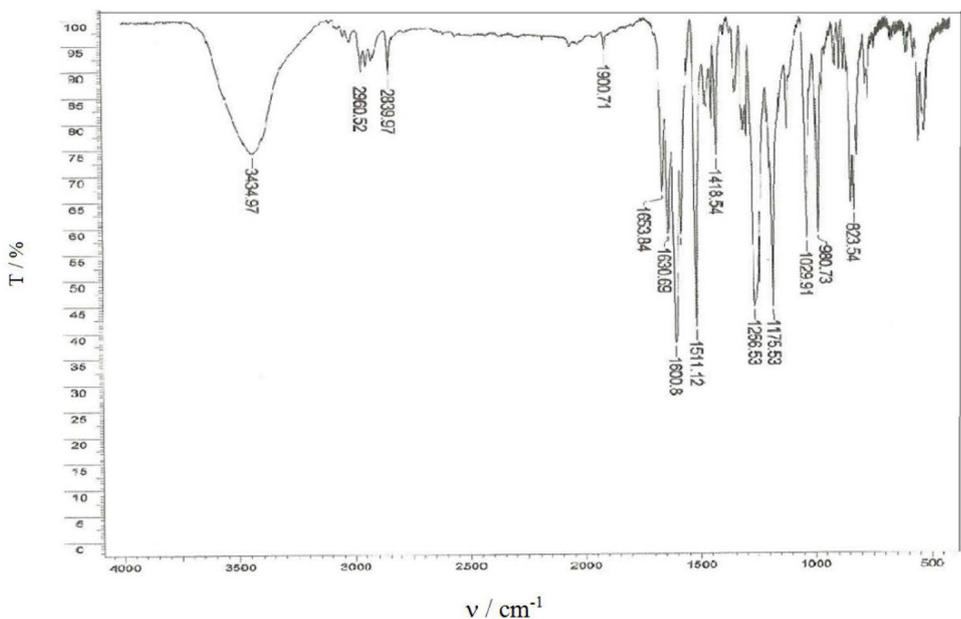
Figure S1. IR spectrum (KBr) of (1*E*,4*E*)-1,5-bis(4-methoxyphenyl)-1,4-pentadien-3-one.
