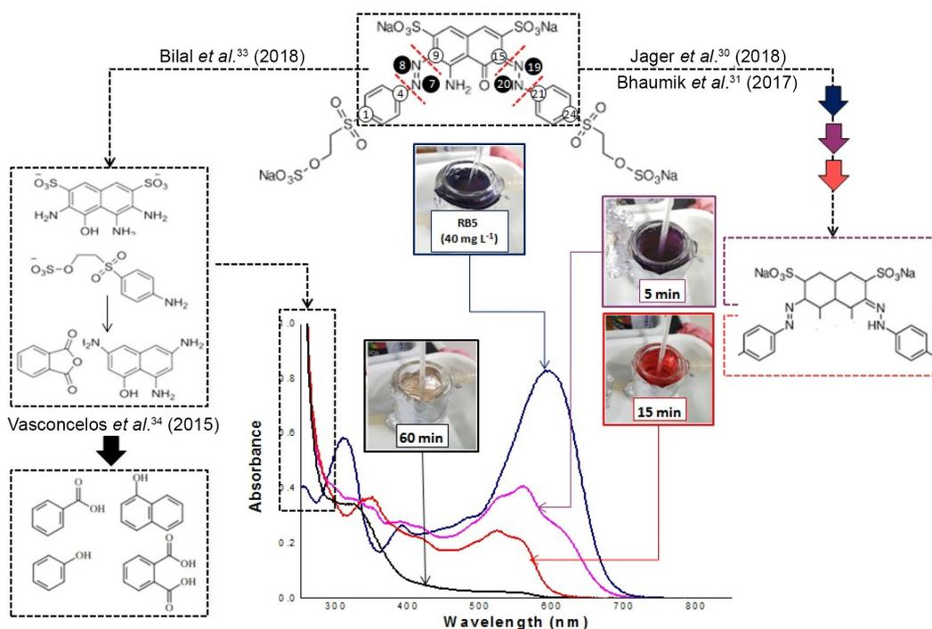
**Figure 2.** Degradation profile and color evolution during the degradation of Reactive Black 5 (40 mg L<sup>-1</sup>) by thermally-activated persulfate (experimental conditions: T = 80 °C, C<sub>ps</sub> = 300 mg L<sup>-1</sup>, pH = 4.0) and possible transient species based on literature background.<sup>30,31,33,34</sup>
