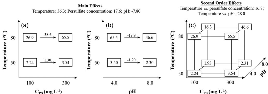
**Figure 1.** Geometric representation of the 2<sup>3</sup> full-factorial design used to evaluate the effects of experimental variables on the degradation of the model dye (Reactive Black 5, C<sub>RB5</sub> = 40.0 mg L<sup>-1</sup>) by thermally-activated persulfate system.
