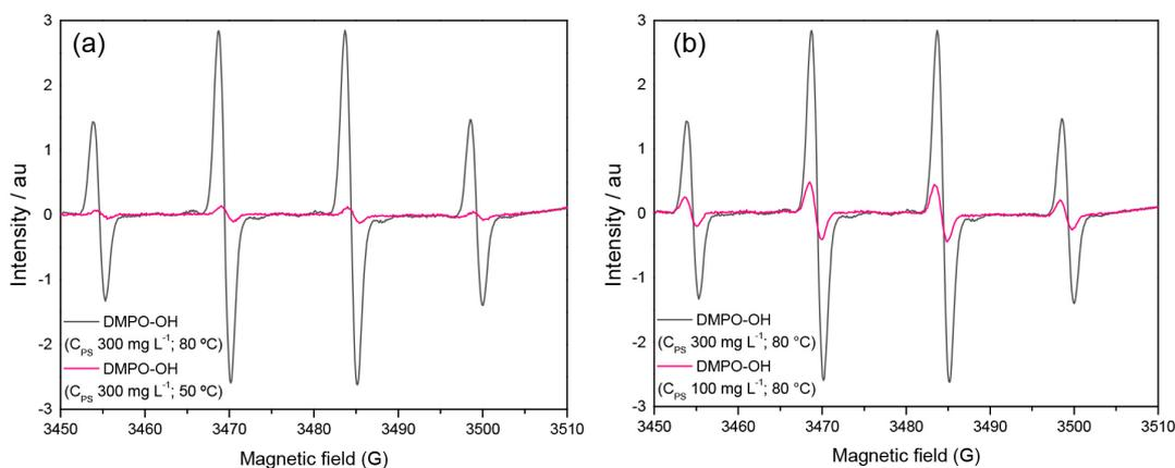
**Figure 4.** EPR spectra of the  $\bullet\text{DMPO-OH}$  adduct acquired in aqueous solution at 298 K. (a) Effect of activation temperature ( $C_{\text{PS}} = 300 \text{ mg L}^{-1}$ ,  $C_{\text{DMPO}} = 20.0 \text{ mM}$ ) and (b) effect of persulfate concentration ( $T = 80.0 \text{ }^\circ\text{C}$ ,  $C_{\text{DMPO}} = 20.0 \text{ mM}$ ).
