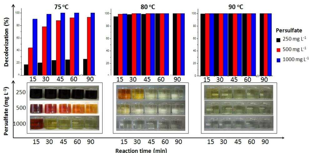
Figure 5. Decolorization of the dyebath by thermally-activated persulfate ( $C_{ps} = 250, 500, \text{ and } 1000 \text{ mg L}^{-1}$ ;  $T = 75.0, 80.0, \text{ and } 90.0 \text{ } ^\circ\text{C}$ ).
