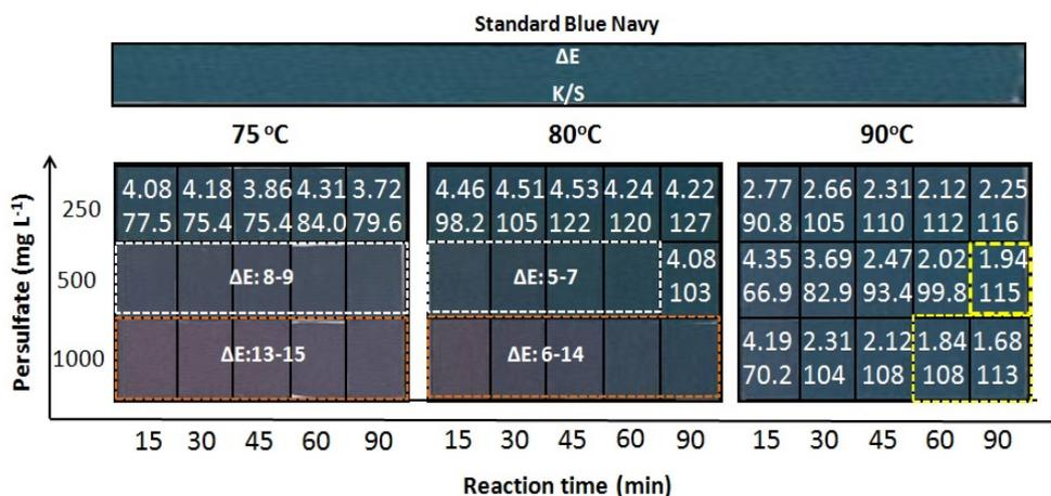
Figure 6. The color difference of fabrics dyed with dyebaths treated by thermally-activated persulfate.
