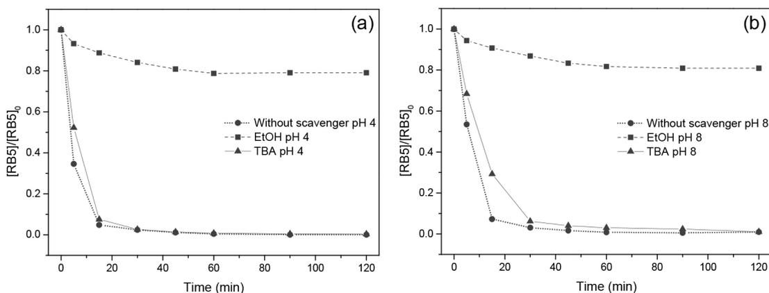
**Figure 3.** Degradation of Reactive Black 5 (40.0 mg L<sup>-1</sup>) by thermally-activated persulfate ( $C_{\text{PS}} = 300 \text{ mg L}^{-1}$ ,  $T = 80.0 \text{ }^{\circ}\text{C}$ ) in the presence and absence of radical scavengers at pH 4.00 (a) and pH 8.00 (b).
