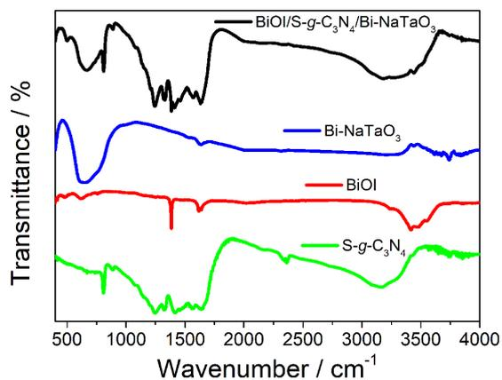
**Figure 2.** FTIR (KBr) spectra of S-*g*-C<sub>3</sub>N<sub>4</sub>, BiOI, Bi-NaTaO<sub>3</sub>, and BiOI/S-*g*-C<sub>3</sub>N<sub>4</sub>/Bi-NaTaO<sub>3</sub>.
