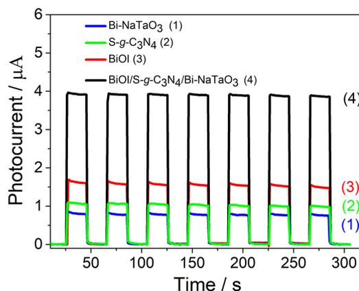
**Figure 5.** Photocurrents obtained for the FTO modified with Bi-NaTaO<sub>3</sub>, S-g-C<sub>3</sub>N<sub>4</sub>, BiOI, and BiOI/S-g-C<sub>3</sub>N<sub>4</sub>/Bi-NaTaO<sub>3</sub> in 5 mmol L<sup>-1</sup> of TBHQ in 0.1 mol L<sup>-1</sup> phosphate buffer (pH = 7) under an applied potential of 0.0 V vs. Ag/AgCl (KCl<sub>Sat</sub>) and incidence of chopped light.
