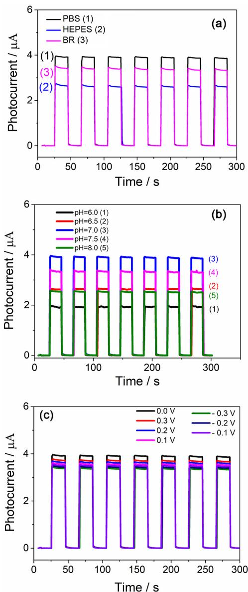
**Figure 7.** Effects of experimental parameters on the photocurrent of the BiOI/S-g-C<sub>3</sub>N<sub>4</sub>/Bi-NaTaO<sub>3</sub>/FTO photoelectrode for 5 mmol L<sup>-1</sup> TBHQ: (a) buffer solution at pH 7.0 and 0.1 mol L<sup>-1</sup>, (b) pH and (c) applied potential. PBS: phosphate buffer solution.
