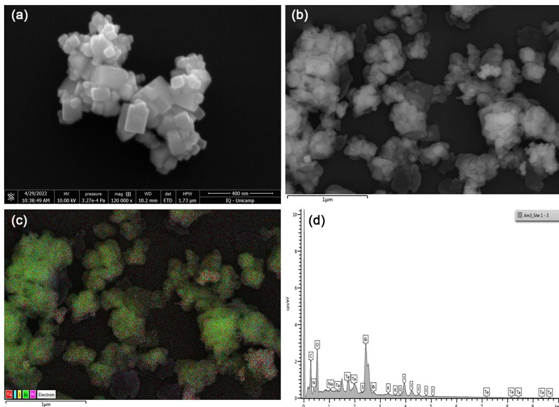
**Figure 4.** SEM images for the Bi-NaTaO<sub>3</sub> perovskite (a), and for the BiOI/S-g-C<sub>3</sub>N<sub>4</sub>/Bi-NaTaO<sub>3</sub> composite (b). Energy dispersive X-ray spectroscopy elemental mapping (c) and EDS spectrum for a sample of the BiOI/S-g-C<sub>3</sub>N<sub>4</sub>/Bi-NaTaO<sub>3</sub> composite (d).
