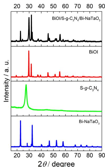
**Figure 1.** XRD patterns of Bi-NaTaO<sub>3</sub>, BiOI, S-g-C<sub>3</sub>N<sub>4</sub>, and BiOI/S-g-C<sub>3</sub>N<sub>4</sub>/Bi-NaTaO<sub>3</sub>.
