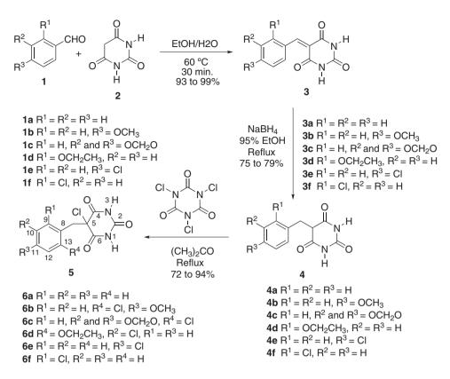
Scheme 1. Synthetic sequence for the preparation of 5-chloro-benzobarbiturates.
