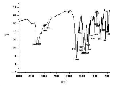
Figure S6. IR spectrum of 6b.
