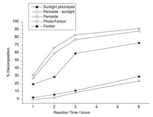
**Figure 2.** Comparison among sunlight photolysis ( $\blacksquare$ ), oxidation using hydrogen peroxide in the presence ( $\bigcirc$ ) and absence ( $\triangle$ ) of sunlight, degradation by Fenton ( $\blacklozenge$ ) and photo-Fenton ( $\bigtriangledown$ ) processes for the degradation of aqueous acetonitrile residues.
