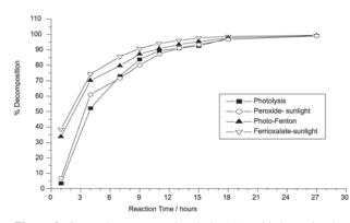
**Figure 3.** Comparison among photolysis  $(\blacksquare)$ , oxidation using hydrogen peroxide under sunlight  $(\bigcirc)$ , photo-Fenton under sunlight  $(\blacktriangle)$  and ferrioxalate under sunlight  $(\bigtriangledown)$  processes for the degradation of aqueous acetonitrile residues.
