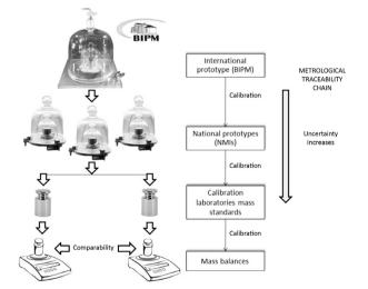
Figure 1. Metrological traceability in calibration laboratories: example for mass calibration.
