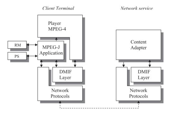
Figure 1: The 3DVEAdapt framework components.
