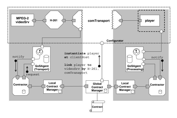
Figure 12: Mapping the VoD application contract in the architectural pattern
