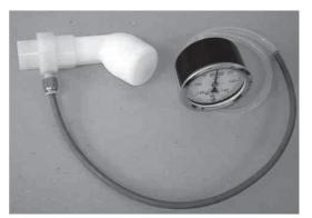
**Figure 1** - Adaptation to allow the vacuum manometer and the Flutter VRP1<sup>®</sup> to be connected in order to measure and record expiratory pressures at each exhalation.
