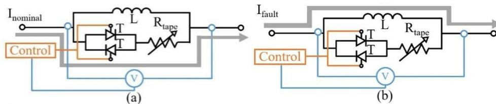
Fig. 1. Simplified hybrid SFCL circuit in (a) the normal operation and (b) during fault conditions.
