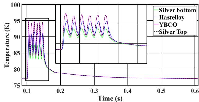
Fig. 12. Temperatures of the superconducting layers - Limiter with emulated mechanical switch.
