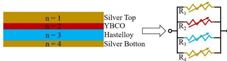
Fig. 2. Cross-section of the tape 2G YBCO and its electrical representation [19], [30], [32].
