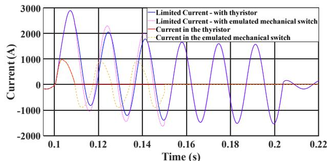
Fig. 13. Limited current using thyristors and emulated mechanic switch.
