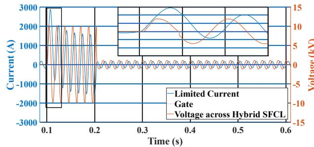
Fig. 10. The controlling relationship between current and voltage.
