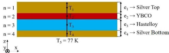
Fig. 4. Temperature variation within a cross-section of the superconducting tape layers. Adapted from [19], [30], [32].
