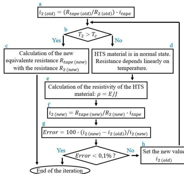
Fig. 3. Flowchart of the iterative process of resistivity and electric current in the superconductor. Adapted from [30], [32].
