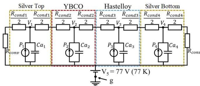
Fig. 5. Thermal-electrical equivalent for the 2G tape. Adapted from [19], [30], [32].
