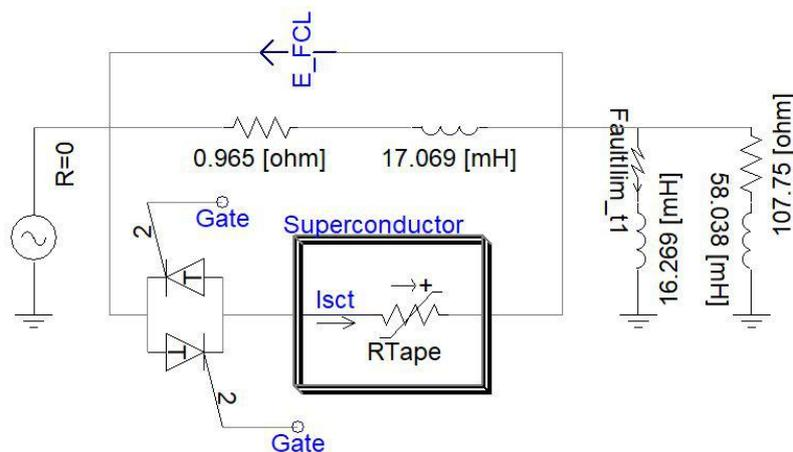
Fig. 6. Proposed Hybrid SFCL simulation in PSCAD/EMTDC software.
