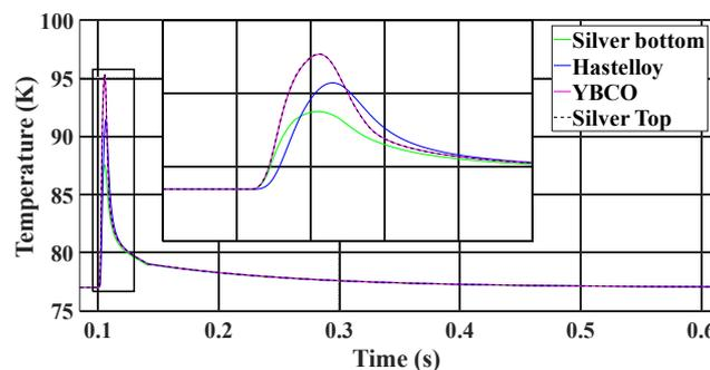
Fig. 11. Temperature rise of each of the superconducting layer - using thyristors.
