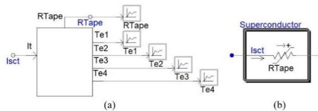
Fig. 7. (a) Component created in PSCAD/EMTDC to calculate the resistance of the superconducting tape and (b) variable resistance.
