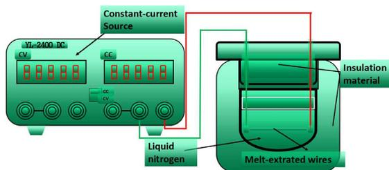
**Figure 1.** Schematic illustration of CJA process with insulation material and the microwire surrounding by nitrogen gap during annealing process.
