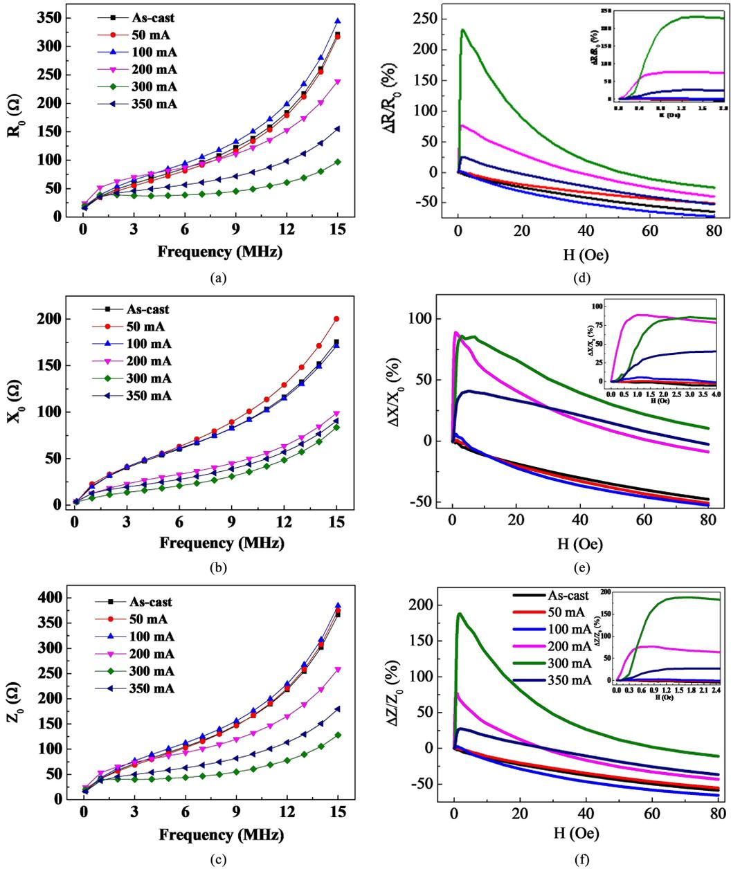
**Figure 3.** Frequency dependence of (a) resistance  $R(H_0)$ , (b) inductive reactance  $X(H_0)$  and (c) impedance  $Z(H_0)$  and field dependence of (d) magneto-resistance ( $\Delta R/R_0$ ), (e) magneto-reactance ( $\Delta X/X_0$ ), and (f) magneto-impedance ( $\Delta Z/Z_0$ ) ratios with annealing current in the range of 0–350 mA. Insets of the magnified peak positions of  $\Delta R/R_0$ ,  $\Delta X/X_0$  and  $\Delta Z/Z_0$  in (d), (e) and (f) respectively.
