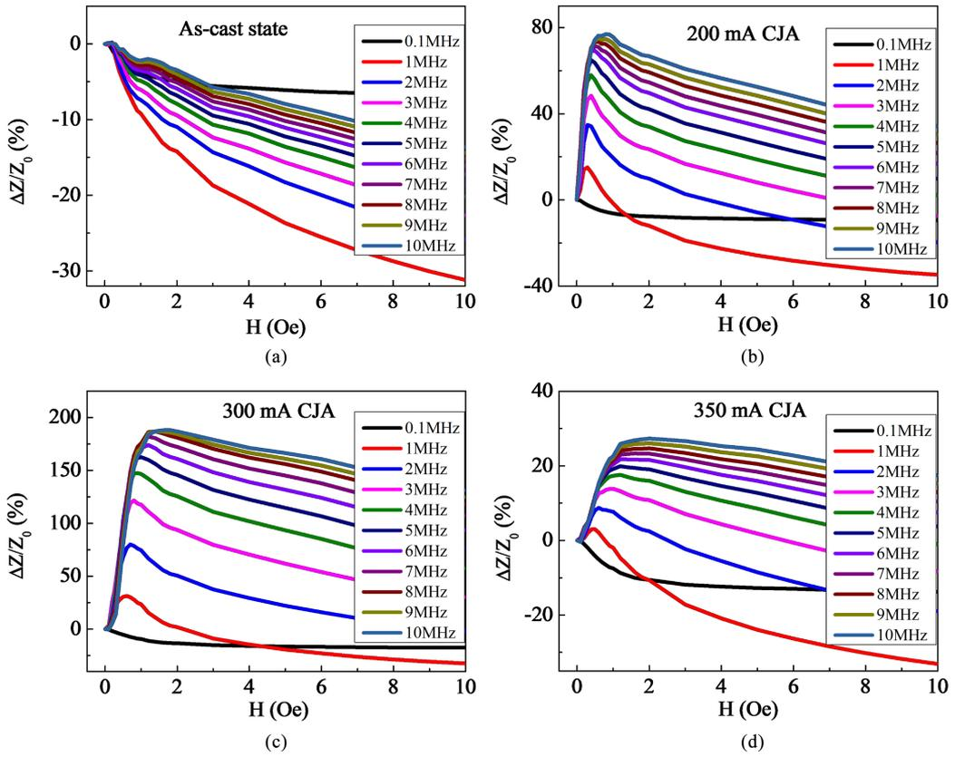
**Figure 2.** Field dependence of GMI curves measured with selected CJA-ed sample for  $t=240$  s. (a) As-cast; (b) 200 mA; (c) 300 mA; (d) 350 mA.
