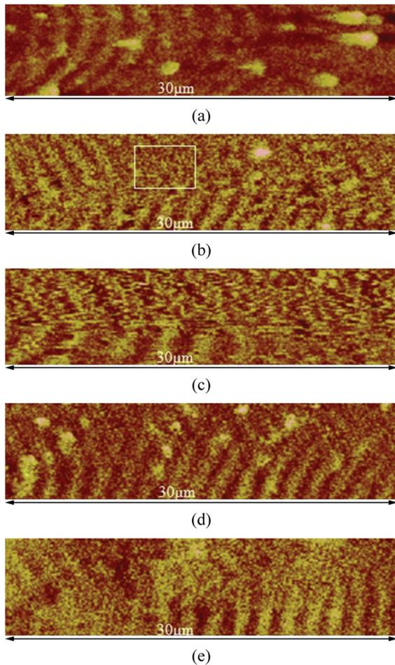
**Figure 4.** Magnetic domain structures of melt-extracted Co-based amorphous wires: (a) as-cast state; (b) 100 mA; (c) 200 mA; (d) 300 mA; (e) 350 mA; Ruler point is axial direction of microwire.
