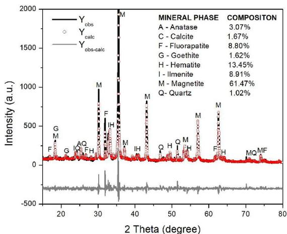
**Figure 1.** X-ray diffractogram of the magnetic tailings obtained from phosphate-rock processing in Alto Paranaíba.
