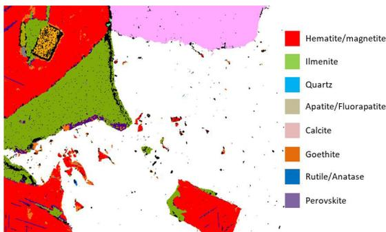
Figure 8. Mineral phase map of phosphate-ore tailings obtained from QEM.
