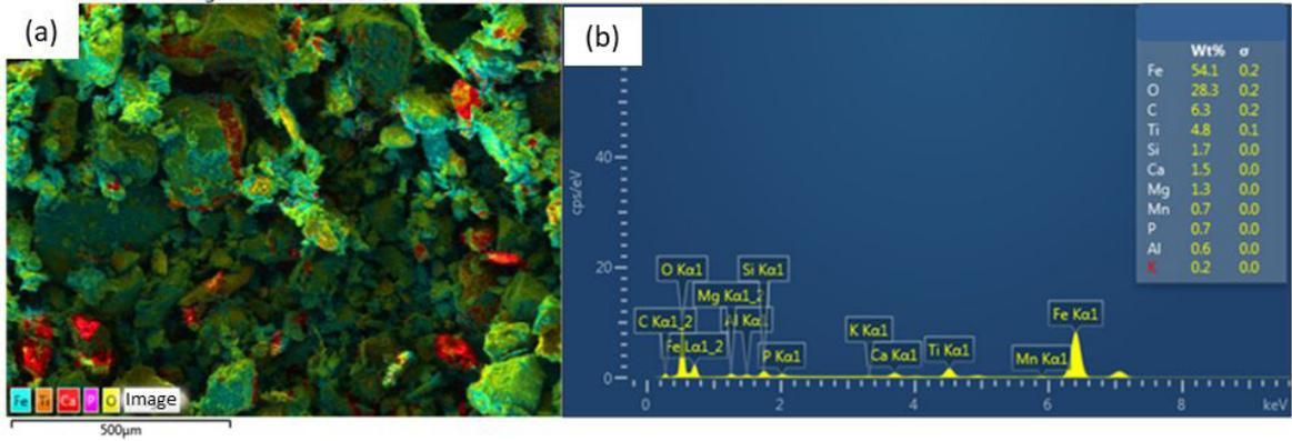
**Figure 4.** (a) Image and (b) dispersive energy spectrum of a magnetic-waste sample obtained from phosphate-rock processing.
