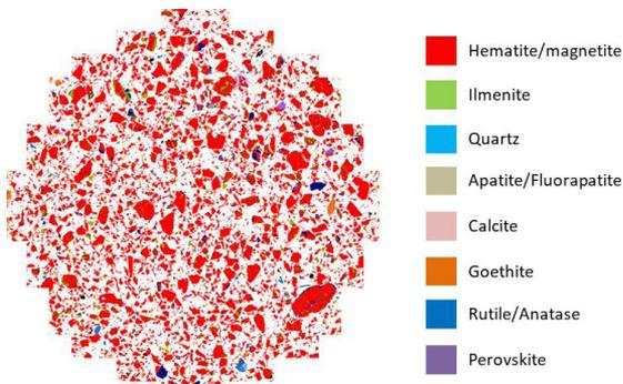
**Figure 3.** Phase map of the ferromagnetic tailings sample using the Quantitative Electronic Microscope (QEM).
