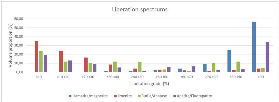
Figure 7. Volume liberation spectrum of the mineral phases of magnetic tailings obtained from phosphate-rock processing.
