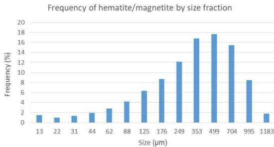
**Figure 6.** Particle size distribution of only hematite/magnetite by size.
