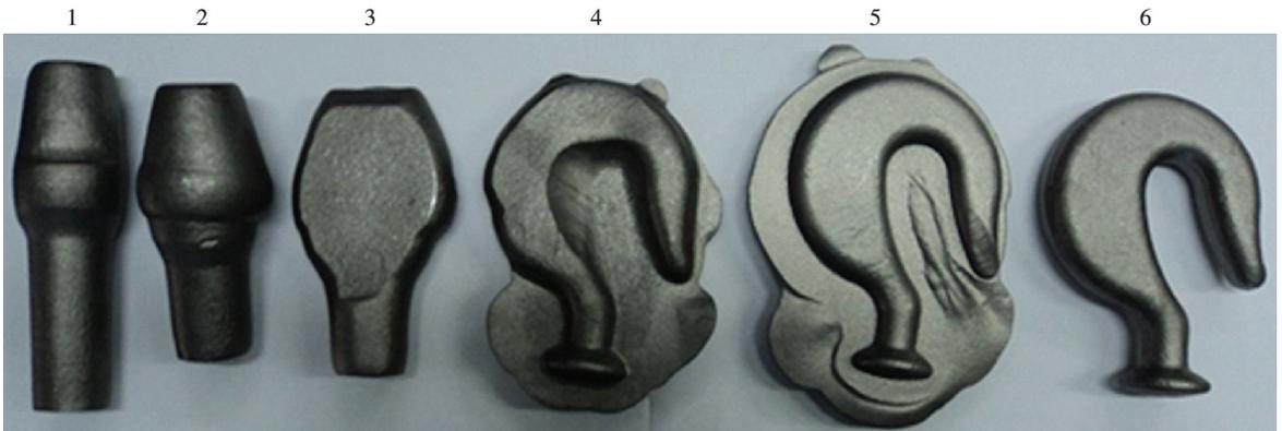
Figure 2. Workpieces after forging stages 1-6 (from left to right): 1-2: upsetting; 3: flattening; 4-5: die-forging; 6 final product after flash removal.
