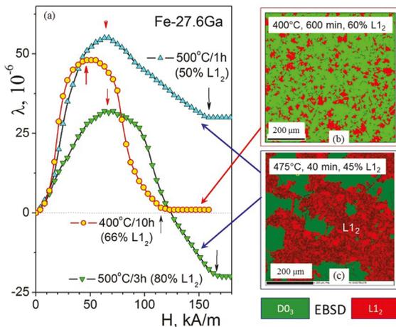
**Figure 4.** Magnetostriction vs applied field and different dispersion of the  $L1_2$  (red color) phase at 400 (fine) and 475/500°C (coarse grains).
