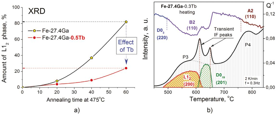
**Figure 7.** (a) Amount of  $L1_2$  phase determined by X-ray analysis after isothermal annealing in the Fe-27.4Ga (yellow circles) and in the Fe-27.4Ga-0.5Tb (red circles) samples; (b) Phase transitions in the Fe-27.4Ga-0.3Tb sample according to the *in situ* neutron diffraction (Intensity, left Y-axis) and TDIF (black curve corresponds to right Y-axis).
