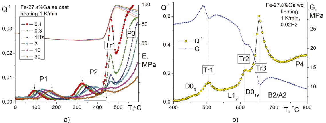
**Figure 1.** TDIF curves measured at heating with 1 K/min rate using bending (up to 600°C, DMA Q800; left figure) and torsion (up to 800°C, inverted pendulum; right figure) vibrations with different frequencies from 0.02 to 30 Hz (see in figures).
