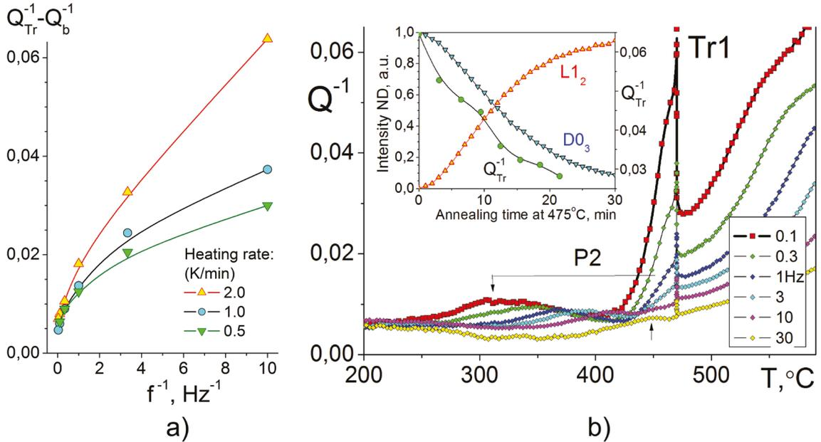
**Figure 3.** a) The Tr1-peak height as a function of inverse frequency for three different heating rates; b) TDIF curve with interrupted heating at 470°C. Inset: The decrease of the Tr1 peak as a function of time of isothermal annealing (green circles) and intensities of neutron diffraction lines from decaying  $D0_3$  phase (blue down triangles) and growing  $L1_2$  phase (red up triangles) under the same conditions.
