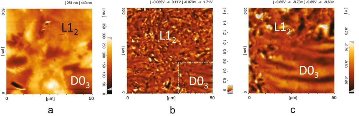
**Figure 5.** Topography (a), low magnification MFM (b), and high magnification MFM (c) images of the Fe-27.8Ga sample annealed at 400 °C for 600 min showing  $D0_3$  (darker contrast) and  $L1_2$  (brighter contrast) phases.
