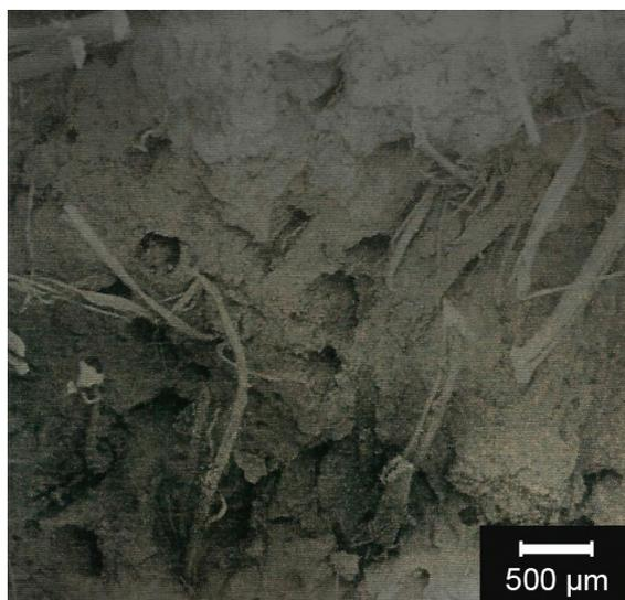
Figure 2. Fracture surface of a 25 mm fiber reinforced bend specimen.
