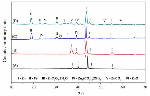
**Figure 6.** XRD diffractograms of the zinc coating untreated and treated by in oxalic acid solution, before and after exposure for 30 days in B100 biodiesel: (A) Coating untreated before exposure; (B) Coating untreated after exposure; (C) Coating treated before exposure; (D) Coating treated after exposure.
