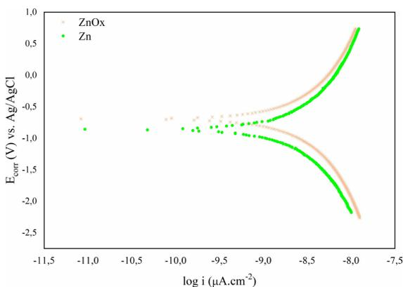
**Figure 2.** Potentiodynamic polarization curves in soybean biodiesel of Zn coating not subject (Zn) and subject to the conversion treatment (ZnOx). The curves were obtained at a temperature of 25 °C, at a sweep rate of 10 mV/s.
