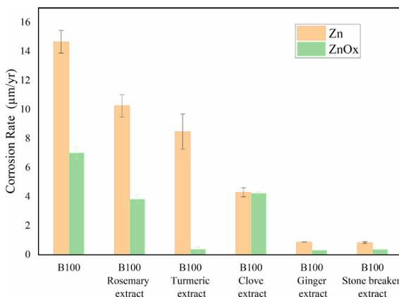
**Figure 3.** Corrosion rate of zinc coatings not subject (Zn) and subject to the conversion treatment (ZnOx). The corrosion rate was determined after 30 days of immersion in B100 biodiesel in the absence and presence of 1000 ppm of different additives.
