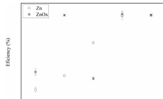
**Figure 4.** Corrosion inhibition efficiency in B100 solution of additives on zinc coating not subject (Zn) and subject to the conversion treatment (ZnOx).
