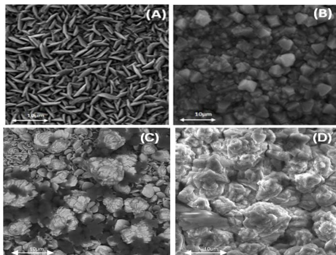
**Figure 7.** SEM micrographs of zinc coatings, untreated and treatment in oxalic solution before and after immersion for 30 days in B100 biodiesel in the absence of additive: (A) untreated before immersion; (B) treated before immersion; (C) untreated after immersion; (D) treated after immersion.
