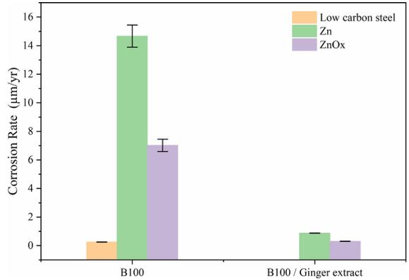
**Figure 5.** Corrosion rate after 30 days of immersion in B100 in the absence and presence of 1000 ppm of extract ginger as an additive. Corrosion rate corresponds to the following samples: low carbon steel; zinc coating subject to the conversion treatment; and Zn coating not subjected to this treatment.
