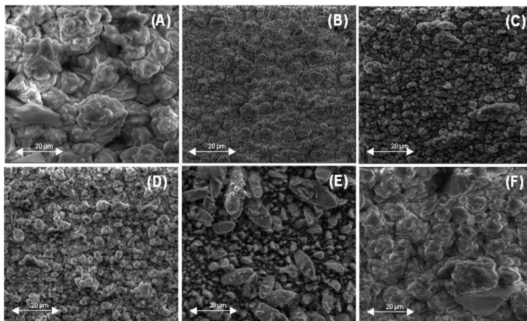
**Figure 8.** SEM micrographs of zinc coatings treatment in oxalic solution and immersion for 30 days in B100 in the absence and presence of 1000 ppm of different additives: (A) absence of additive; (B) presence of turmeric extract; (C) presence of ginger extract; (D) presence of stone breaker extract; (E) clove extract; (F) rosemary extract.
