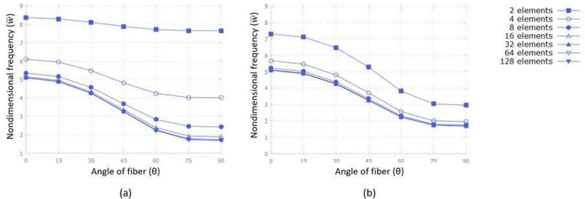
Figure 5. (a) Second frequency for different ply fiber directions for the clamped-free (CF) beam computed using the parasitic shear finite element model; (b) Second frequency for different ply fiber directions for the clamped-free (CF) beam computed using the corrected finite element model.
