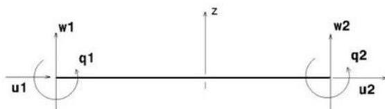
Figure 2. Two-node beam finite element.
