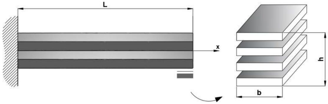
Figure 9. Clamped-Supported (CS) laminated composite beam problem model.
