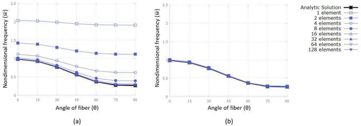
Figure 4. (a) First frequency for different ply fiber directions for the clamped-free (CF) beam computed using the parasitic shear finite element model; (b) First frequency for different ply fiber directions for the clamped-free (CF) beam computed using the corrected finite element model.
