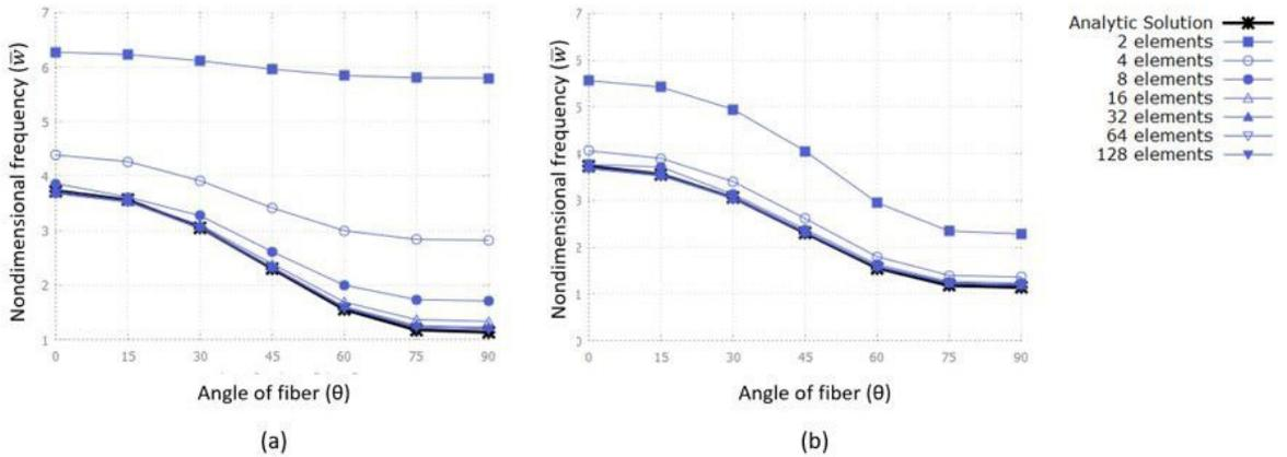
Figure 10. (a) First frequency for different ply fiber directions for the clamped-free (CS) beam computed using the parasitic shear finite element model; (b) First frequency for different ply fiber directions for the clamped-free (CS) beam computed using the corrected finite element model.
