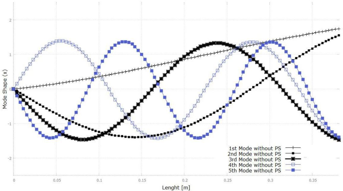
**Figure 12.** First five transversal mode shapes of the clamped-free (CF) beam computed using the parasitic shear finite element model.
