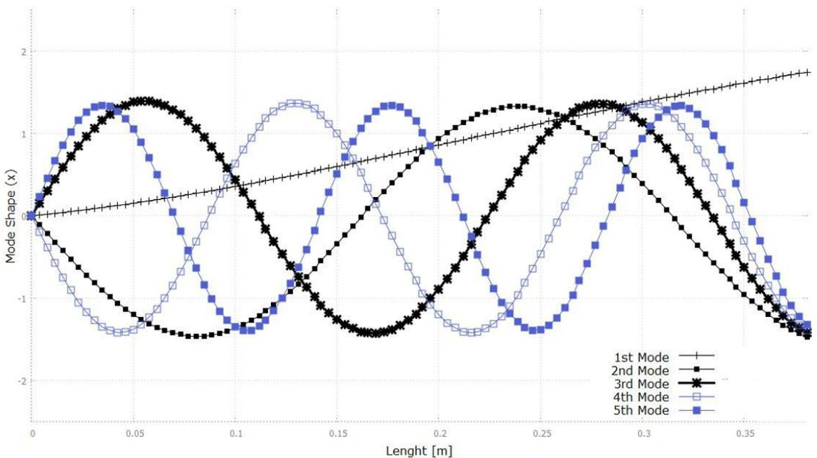
**Figure 11.** First five transversal mode shapes of the clamped-free (CF) beam computed using the corrected finite element model.
