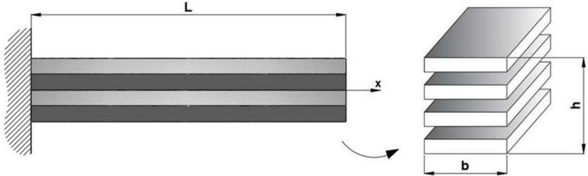
Figure 3. Clamped-Free (CF) laminated composite beam problem model.
