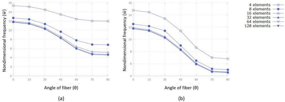
**Figure 6.** (a) Third frequency for different ply fiber directions for the clamped-free (CF) beam computed using the parasitic shear finite element model; (b) Third frequency for different ply fiber directions for the clamped-free (CF) beam computed using the corrected finite element model.
