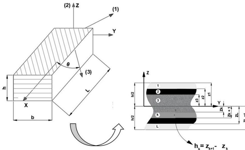
Figure 1. Geometry of a laminated composite beam.
