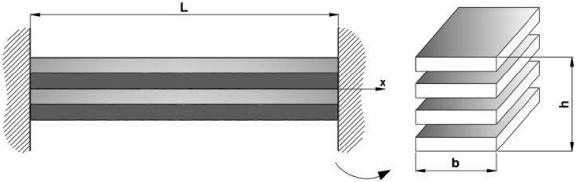
Figure 7. Clamped-Clamped (CC) laminated composite beam problem model.
