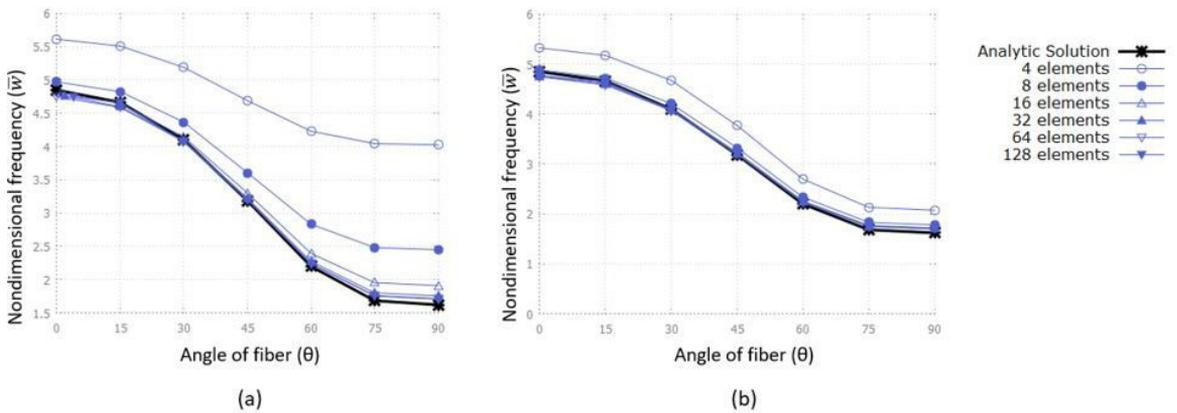
Figure 8. (a) First frequency for different ply fiber directions for the clamped-free (CC) beam computed using the parasitic shear finite element model; (b) First frequency for different ply fiber directions for the clamped-free (CC) beam computed using the corrected finite element model.
