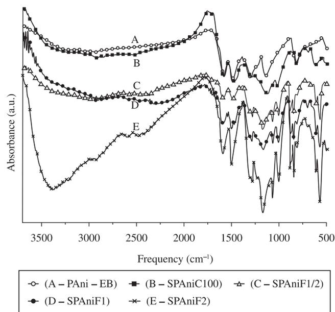
**Figure 1.** PANi-EB and PANi synthesized with both acids FT-IR spectra.
