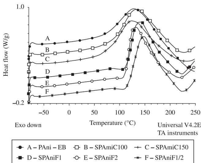
Figure 3. PANi-EB and PANi synthesized with both acids DSC curves.
