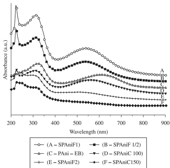
Figure 2. PANi-EB and PANi synthesized with both acids UV-Vis. Spectra.
