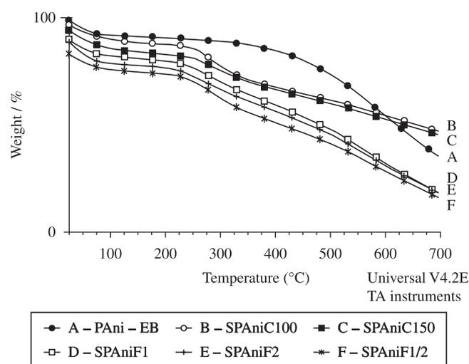
**Figure 4.** PANi-EB and PANi synthesized with both acids TG curves.
