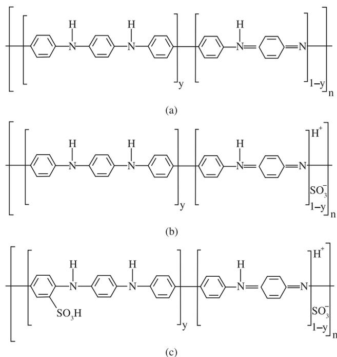
**Figure 6.** Schematic representation of the suggested structure for: a) PAni-EB; b) protonated PAni; and c) protonated and sulfonated PAni.
