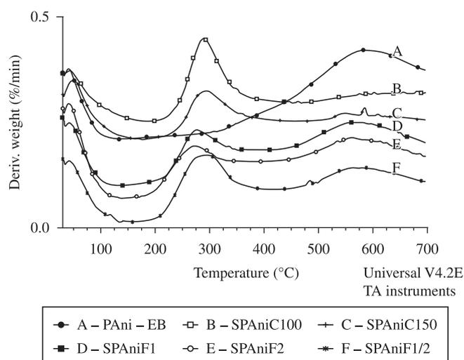
**Figure 5.** PANi-EB and PANi synthesized with both acids DTG curves.
