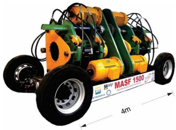
Figure 2. Welding machine, MASF 1500.
