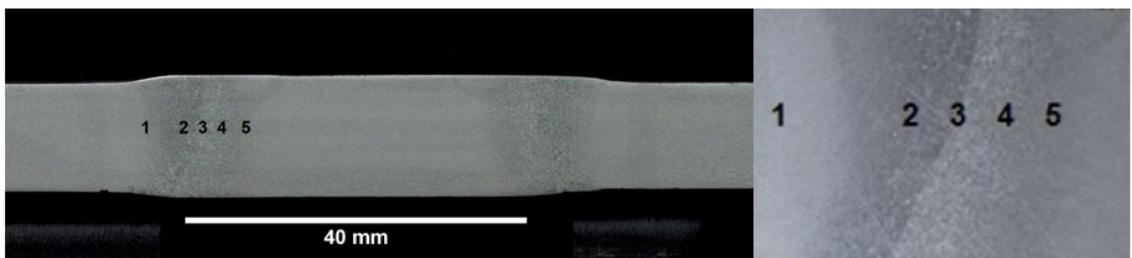
**Figure 4.** Microstructural sections of the welded joint: 1 – pipe HAZ; 2 – pipe TMAZ; 3 – pipe/ring interface; 4 – ring TMAZ and 5 – ring HAZ.
