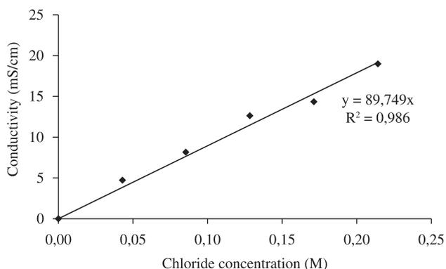
**Figure 3.** Experimental correlation between conductivity (at 25 °C) and chloride concentration in the anolyte chamber initially containing distilled water.
