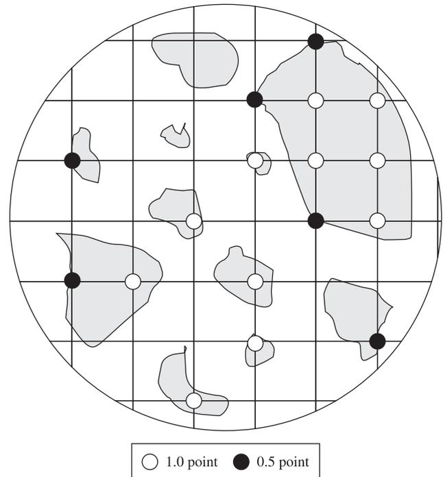
**Figure 1.** Process of sample selection and component quantification for chloride migration tests (in gray, the “gravel phase”); grid nodes inside the phase (in red) correspond to 1, while boundary intersection points (in black) correspond to 0.5.
