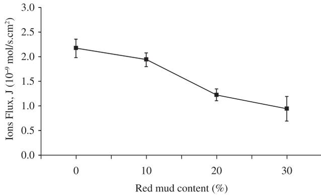
**Figure 11.** Chloride ion flow as a function of red mud content in concrete cured for 28 days, estimated from migration tests.
