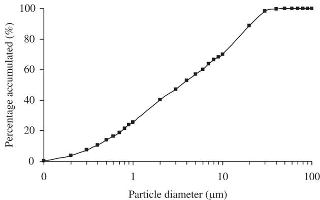
**Figure 4.** Particle size distribution of the dry red mud.
