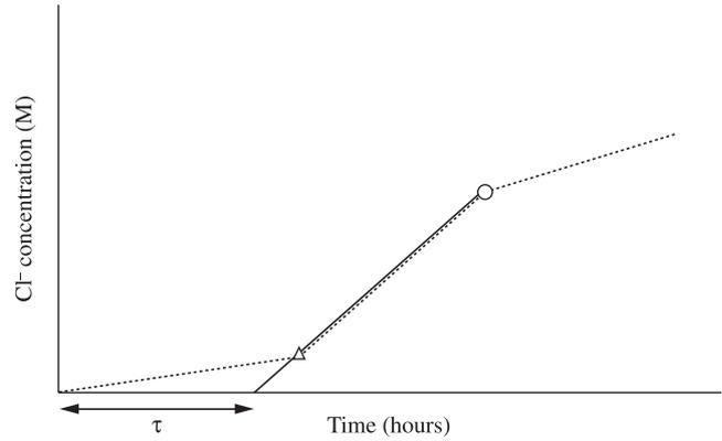
**Figure 9.** Experimental determination of the time lag ( $\tau$ ); onset ( $\Delta$ ) and end (O) of the steady-state diffusion stage, with a diffusion coefficient of  $D_s$ .
