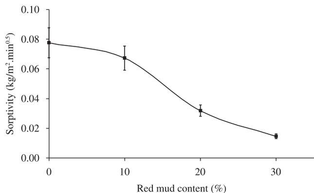
**Figure 15.** Water absorption of concrete specimens as a function of red mud content.
