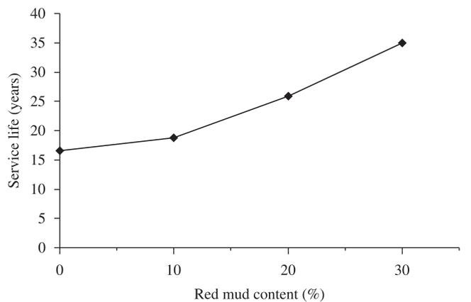
**Figure 14.** Correlation between estimated service life and red mud content in concrete, estimated from a chloride penetration depth of 4 cm depth in the structure.
