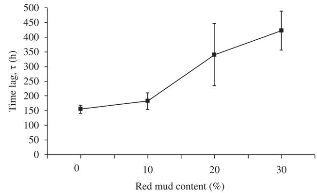
**Figure 10.** Time lag estimated from chloride migration tests as a function of red mud content in concrete cured for 28 days.
