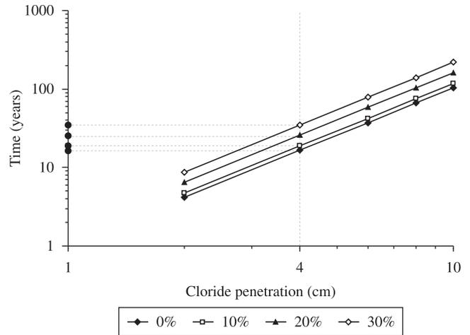
**Figure 13.** Correlation between time and depth of chloride penetration in concrete containing different amounts of red mud (to reach 0.4% Cl<sup>-</sup> per weight of cement).
