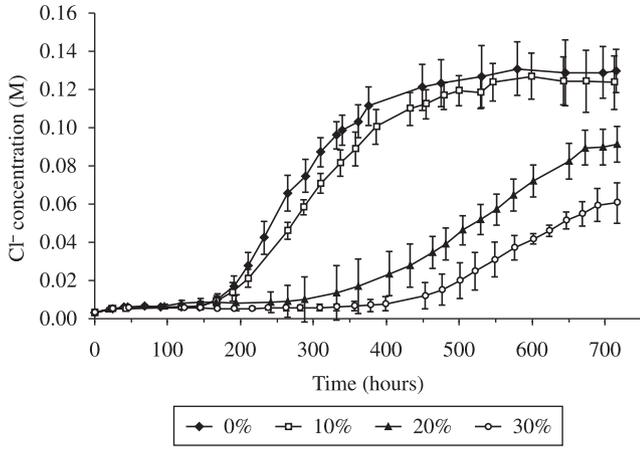
**Figure 8.** Evolution of Cl<sup>-</sup> concentration in the anolyte chamber of a migration test cell over time, based on samples of concrete containing different amounts of red mud (0-30%).
