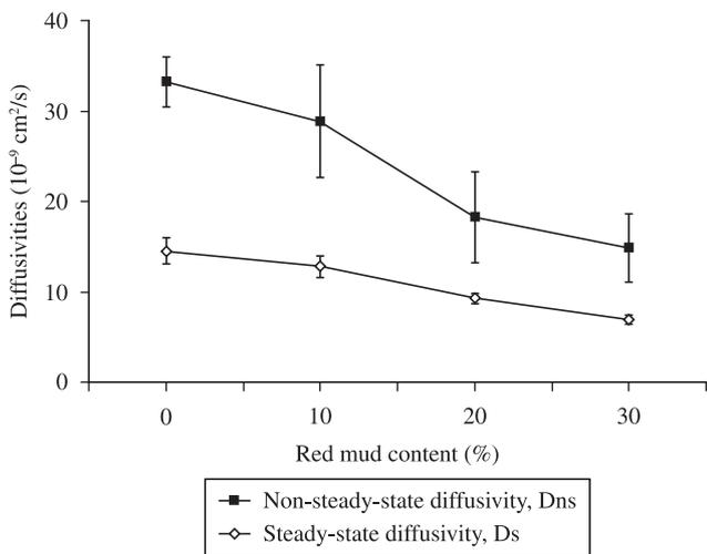
**Figure 12.** Steady-state and nonsteady-state diffusion coefficients of chloride ions as a function of red mud content in concretes cured for 28 days, estimated from migration tests.
