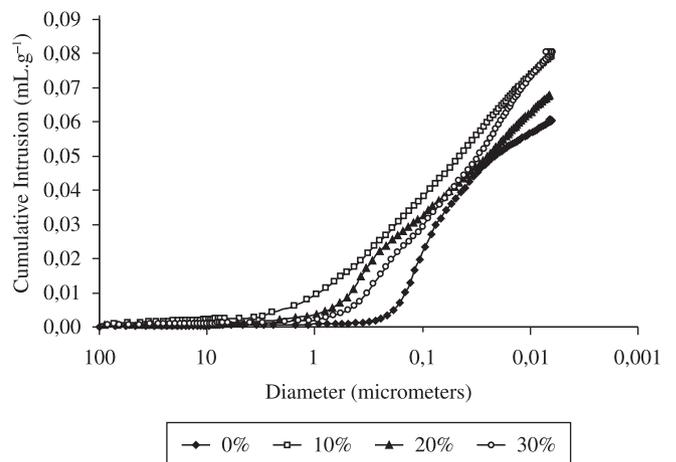
**Figure 7.** Change in the cumulative porosity of concrete with different red mud contents (0-30%) after 28 days of curing.
