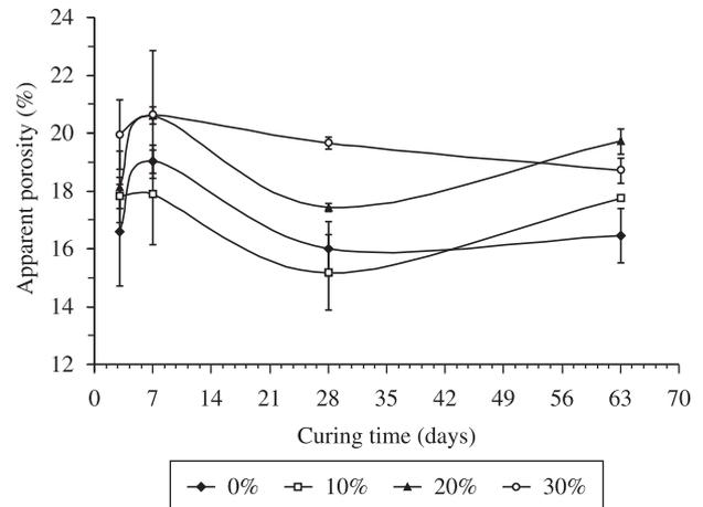
**Figure 6.** Apparent porosity of concrete containing red mud as a function of curing time.
