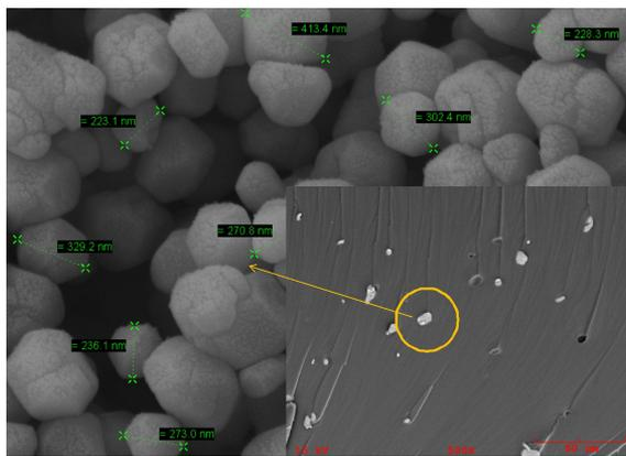
**Figure 3.** SEM micrographs of the photocured materials containing AgNPs.
