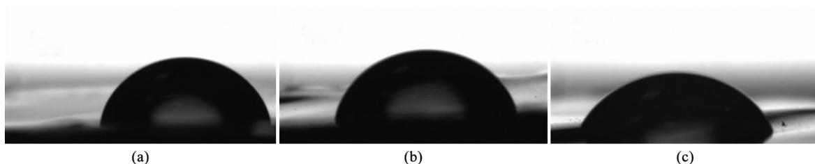
**Figure 6.** Contact angle images of water drop on (a) CF, (b) UA-1AgNPs, and (c) UA-10AgNPs.
