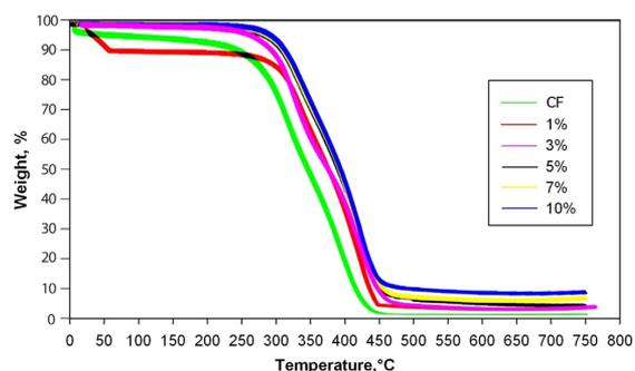
**Figure 4.** TGA spectra of photocured materials.
