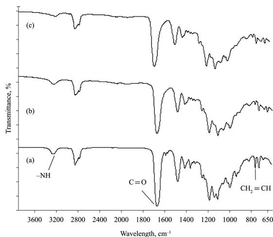
**Figure 2.** FTIR spectra of (a) urethane acrylate oligomer, (b) CF, and (c) UA -10 AgNPs.
