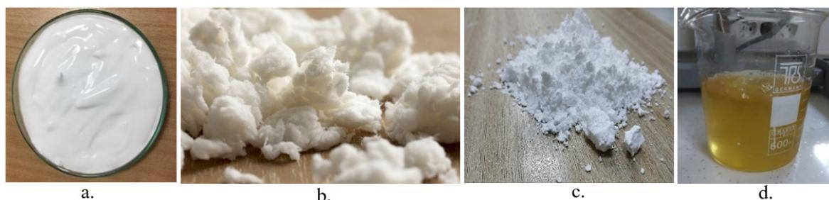
**Figure 1.** Materials used in foam production a. PVAc, b. Bleached kraft pulp, c. Zinc borate, d. Water-soluble chitosan.
