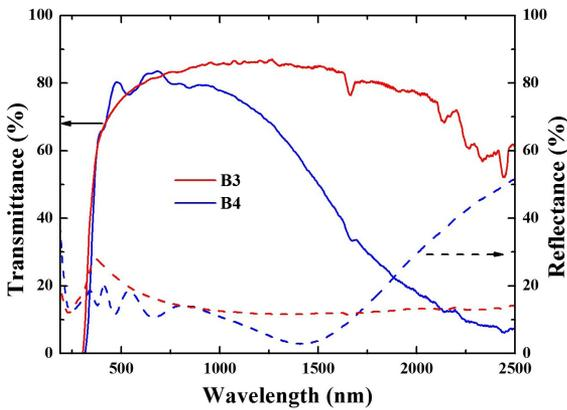
**Figure 5.** Transmittance and reflectance spectra of AZO/PET films deposited under the conditions of sample B2 (PMS and  $d_{r-s}=4\text{cm}$ ) for 5 min (B3) and 30 min (B4).
