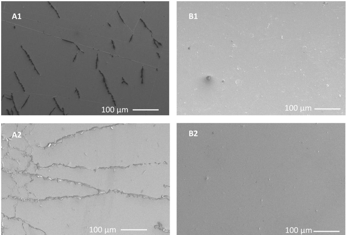
**Figure 3.** Micrographs (obtained by SEM) of AZO/PET films deposited by RF and PMS, with target-substrate distances of 5 and 4 cm. For the films deposited using RF, the presence of cracks is evident, which affects the adhesion to the substrate and the electrical conductivity of the AZO film.
