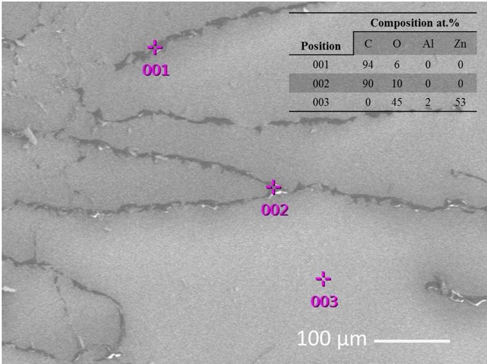
**Figure 4.** Scanning electron micrograph of the AZO/PET films deposited by RF (sample A2). Three positions are indicated where EDS measurements were made. The 001 and 002 positions, which are above cracks, exhibit high concentrations of C, owing to the PET substrate. In contrast, at position 003 only Zn, O and Al, which originate from AZO, are detected.
