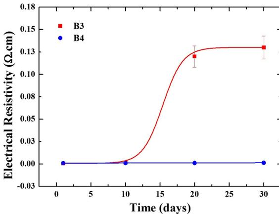
**Figure 6.** Electrical resistivity of the AZO films obtained using PMS as a function of ageing time.
