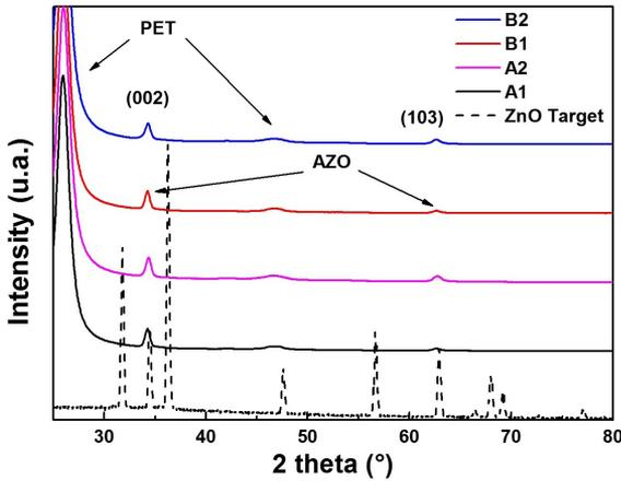
**Figure 2.** X-ray diffractogram of bulk ZnO bulk and of the AZO films deposited on PET. The arrows indicate the DRX peaks of the PET substrate and the (002) and (103) planes of the AZO films.
