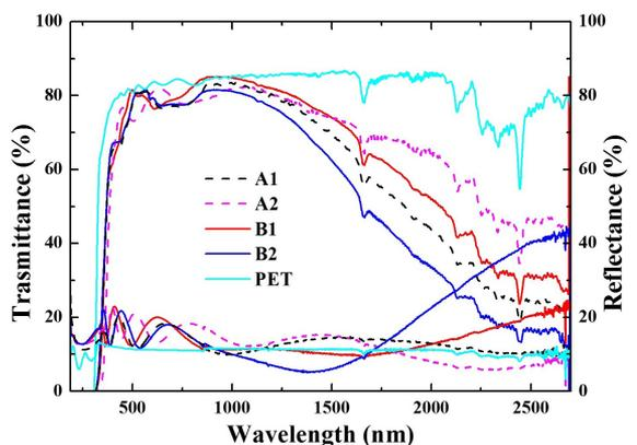
**Figure 1.** Optical transmittance and reflectance spectra of the PET substrate and the AZO/PET samples described in Table 1.
