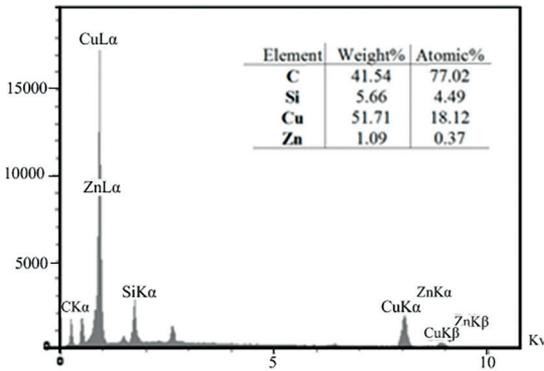
**Figure 4:** SEM images of the intermetallic compounds in the 3-pass FSPed specimen and EDX result.
