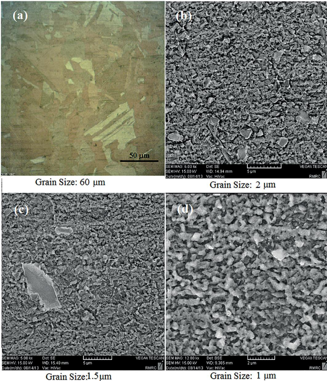
**Figure 6:** (a) Optical microscopy of the base metal and (b-d) SEM images of the 1-, 2- and 3-pass FSPed composites, respectively.
