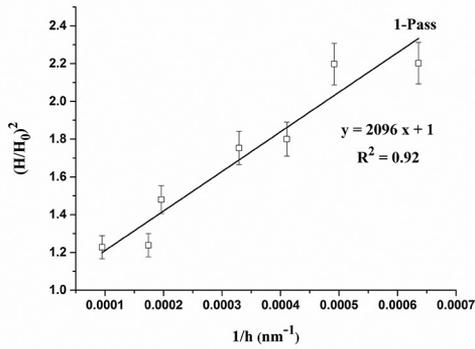
**Figure 7:** Fitting of Eq.(1) to the microhardness data of 1-pass FSPed composite.
