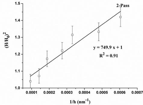
**Figure 8:** Fitting of Eq.(1) to the microhardness data of 2-pass FSPed composite.
