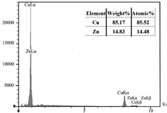
**Figure 2:** SEM images of the intermetallic compounds in the 1-pass FSPed specimen and EDX result.
