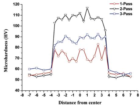
**Figure 10:** Microhardness values of the 1-, 2- and 3-pass FSPed composites.
