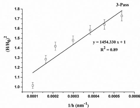
**Figure 9:** Fitting of Eq.(1) to the microhardness data of 3-pass FSPed composite.
