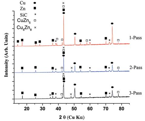
**Figure 5:** X ray diffraction of the Cu-SiC/Zn composites
