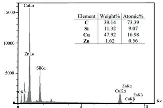
**Figure 3:** SEM images of the intermetallic compounds in the 2-pass FSPed specimen and EDX result.
