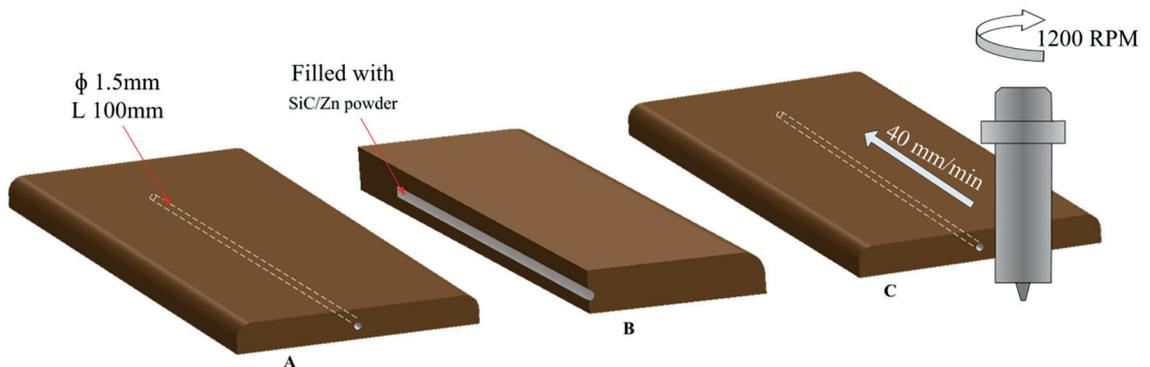
**Figure 1:** Schematic of the friction stir processing (a) drilling the hole in the specimen, (b) compressing the fillers into the hole and (c) plunging the tool into the plate.
