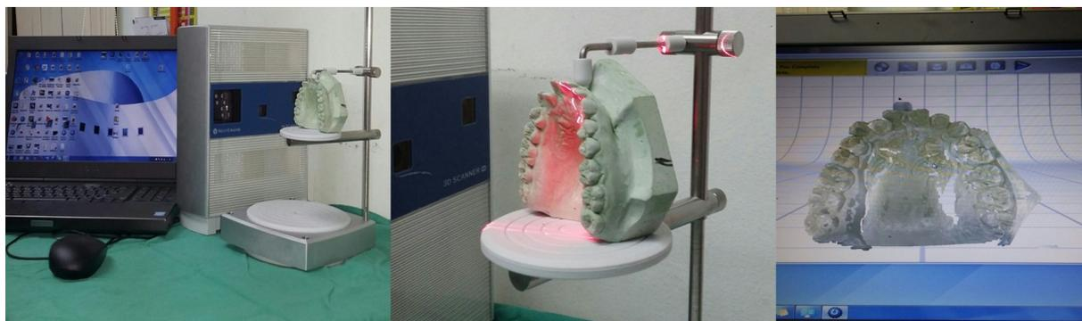
**Figure 1. Conversion of the dental cast into Laser Scanned 3D dental models using Next Engine laser scanner.**
