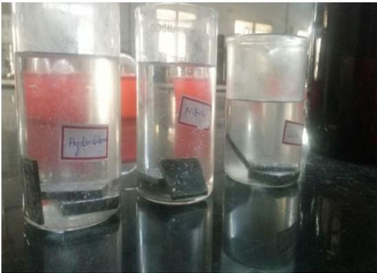
Figure 3. Corrosion test – specimen immersed in acid solution.
