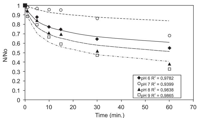
**Figure 2.** Kinetics of *Escherichia coli* inactivation using different initial pH values ( $[H_2O_2]_0 = 100$  mg/L; ◆ pH 6, ○ pH 7, ▲ pH 8, □ pH 9; symbols: experimental; lines: simulation)
