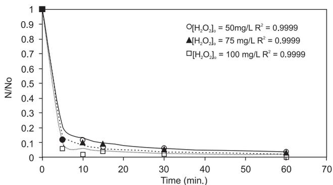
**Figure 1.** Kinetics of inactivation of *Escherichia coli* using different initial  $H_2O_2$  concentrations, pH = 5.6 (○ 50 mg/L, ▲ 75 mg/L, ■ 100 mg/L; symbols: experimental results; lines: simulation)
