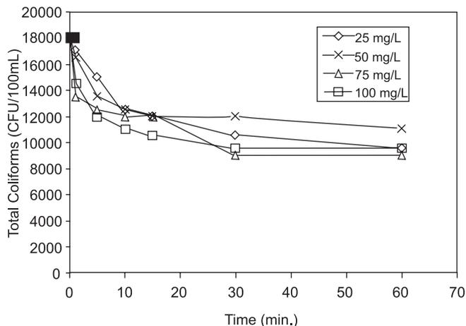
**Figure 4.** Inactivation kinetics of total coliforms in treated domestic sewage using different initial  $H_2O_2$  concentrations at pH = 7.5 (◇ 25 mg/L, × 50 mg/L, △ 75 mg/L, □ 100 mg/L)
