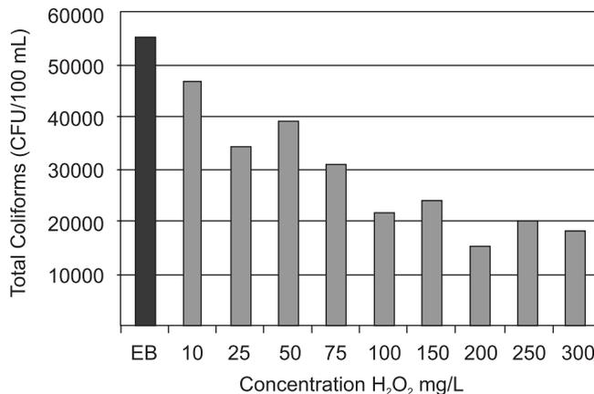
**Figure 3.** Inactivation of total coliforms using different initial  $H_2O_2$  concentrations with a contact time of 10 min (TDS = treated domestic sewage with higher coliform count)
