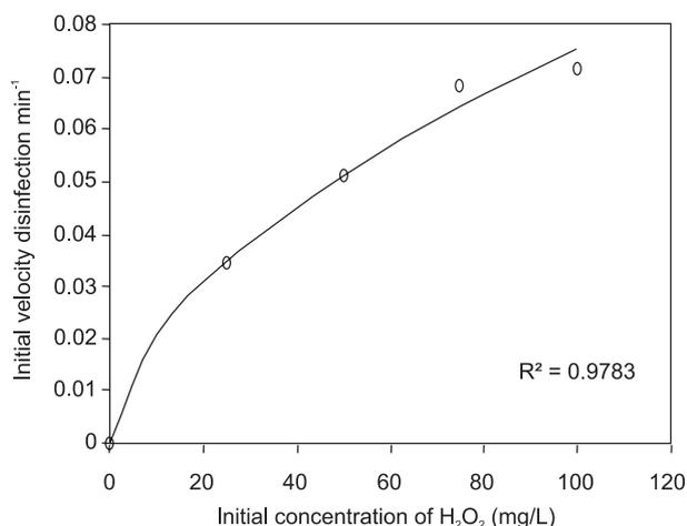
**Figure 5.** Initial inactivation rate of coliforms versus initial concentration of H<sub>2</sub>O<sub>2</sub>. (Points: experimental, line: fit of the dependence of the initial concentration of hydrogen peroxide to the *n*-th power, *n* = 0.56)
