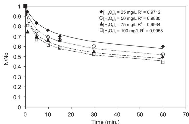
**Figure 6.** Inactivation kinetics of total coliforms in treated domestic sewage using different initial H<sub>2</sub>O<sub>2</sub> concentrations (◆ 25mg/L, ○ 50 mg/L, ▲ 75 mg/L, □ 100 mg/L; symbols: experimental; lines: simulation)
