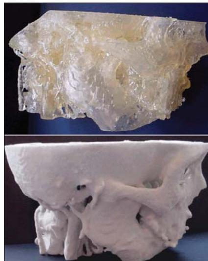
**Figure 5.** Prototypes constructed by the SLA (above) and SLS (below) processes based on a same tomographic data set. Note that the SLA prototype translucence makes the surface visualization difficult.
