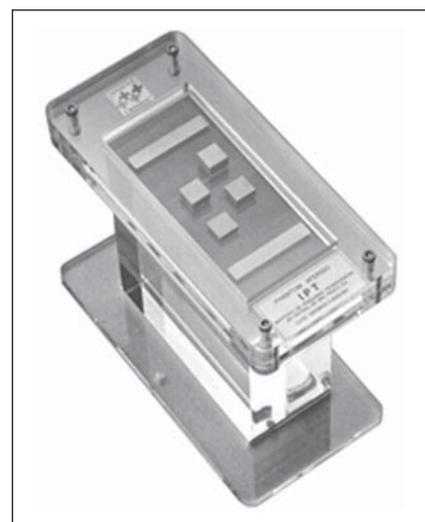
**Figure 1.** Cromox<sup>®</sup> reference phantom in bone absorptiometry constructed with bone specimens measured in the IPT metrology laboratory, and utilized for Cromox<sup>®</sup> devices calibration.
