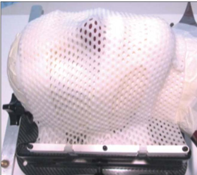
**Figure 2.** ART-210 head phantom properly positioned on the support base, with the set of frameless masks adequately molded to its cranial surface.
