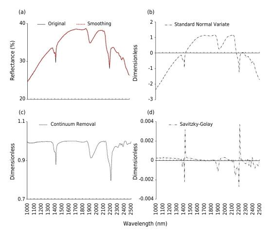
**Figure 2.** Median of spectral curves preprocessed using smoothing (a), standard normal variate (b), continuum removal (c), and Savitzky-Golay derivative (d) approaches.
