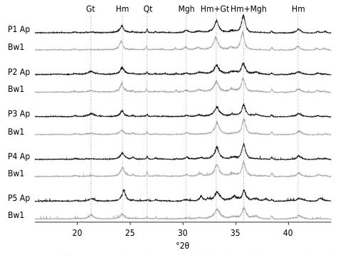
**Figure 2.** X ray diffractograms of powder samples of the iron oxide concentration, showing the variation in the position of the reflections of goethite (Gt), hematite (Hm), quartz (Qt), and maghemite (Mgh) in the Ap and Bw1 horizons of the five studied profiles. P1: Haplic Ferralsol (Dystric, Clayic); P2: Haplic Ferralsol (Dystric, Clayic); P3: Rhodic Eutric Nitisol (Ochric); P4: Rhodic Ferralsol (Dystric, Clayic); P5: Rhodic Ferralsol (Eutric, Clayic).
