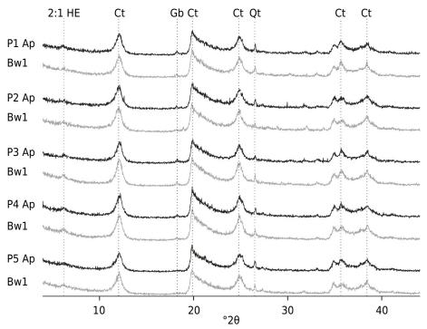
**Figure 3.** X ray diffractograms patterns of powder of iron-free samples, showing the variation in the position of reflections of kaolinite (Ct), gibbsite (Gb), quartz (Qt) and 2: 1 HE in the Ap and Bw1 horizons of the five profiles. P1: Haplic Ferralsol (Dystric, Clayic); P2: Haplic Ferralsol (Dystric, Clayic); P3: Rhodic Eutric Nitisol (Ochric); P4: Rhodic Ferralsol (Dystric, Clayic); P5: Rhodic Ferralsol (Eutric, Clayic).
