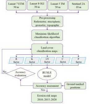
R-annual rainfall-runoff erosivity factor, K-soil erodibility factor, LS-the combination of the slope length and steepness factors, C-cover and management factors, P-support practices factor, and RUSLE-revised universal soil loss equation Figure 2. Flowchart of the image processing procedures used
