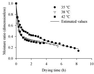
Figure 2. Experimental values and values estimated by the Two Terms model for moisture ratio as a function of drying time of 'Cabacinha' pepper seeds
