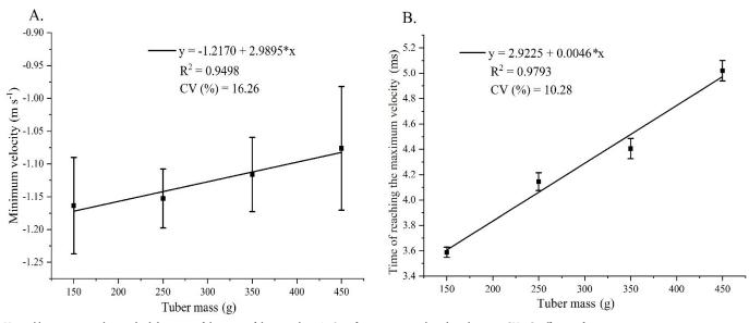
Vertical bars represent the standard deviation of the mean of the ten values. \* - Significant at  $p \le 0.05$  based on the t test; CV - Coefficient of variation **Figure 5.** Relationship between the minimum velocity and tuber mass (A), and time of reaching the maximum velocity and the tuber mass (B) after potato impacted with rod
