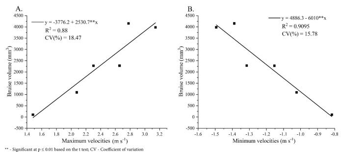
**Figure 6.** Relationship between the maximum velocities and bruise volume (A) and minimum velocities and bruise volume (B) after potato impacted with rod
