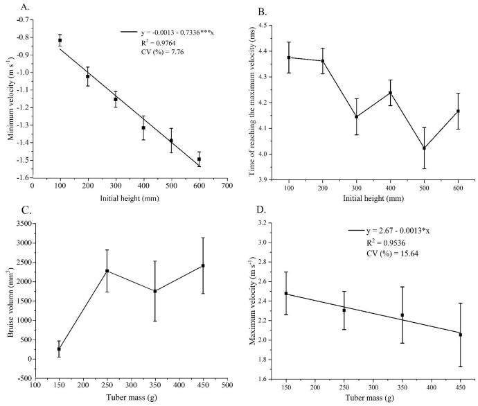
Vertical bars represent the standard deviation of the mean of the ten values. \* - Significant at  $p \le 0.05$ ; \*\*\* - Significant at  $p \le 0.001$  based on the t test; CV - Coefficient of variation **Figure 4.** Relationship between minimum velocity and potato initial height (A), time of reaching the maximum velocity and potato initial height (B), bruise volume and tuber mass (C), and maximum velocity and tuber mass (D)
