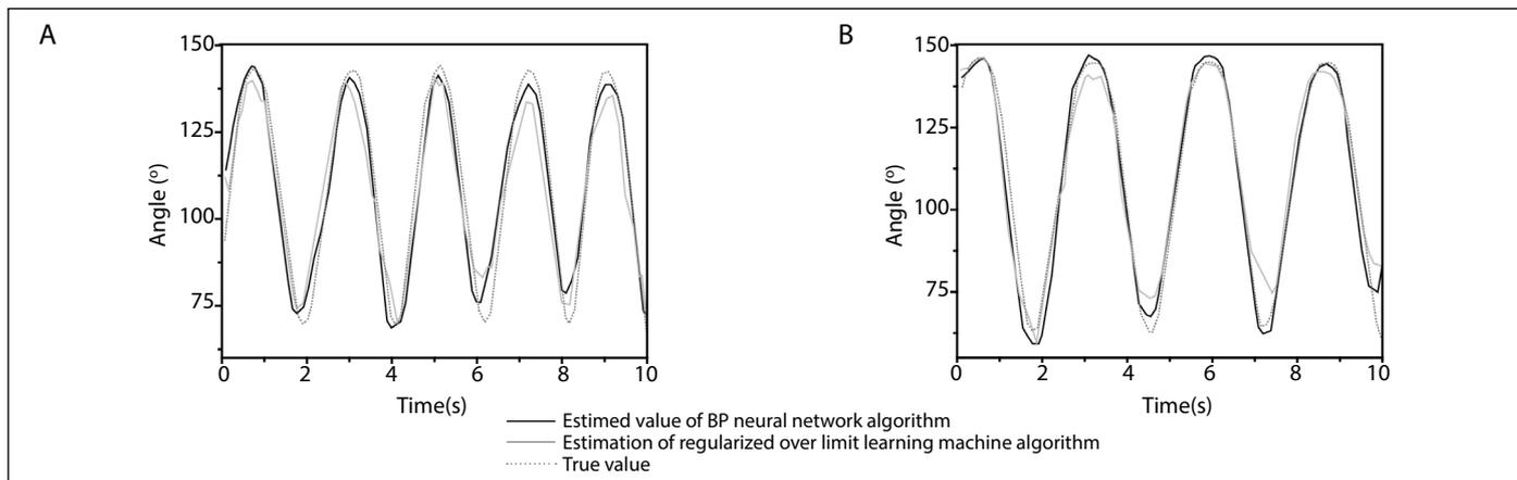
**Figure 3.** Comparison results of regularized over-limit learning machine algorithm and BP neural network algorithm (A shows the result of the indicator prediction model under the knee flexion and extension mode; B shows the result of the indicator prediction model under the squat mode).
