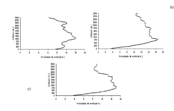
Figure 2 - Vertical profiles of speed of the wind for the days: (a) 04/21/02 at 18UTC, (b) 04/22/02 to the 00UTC and (c) 04/22/02 at 06UTC.
