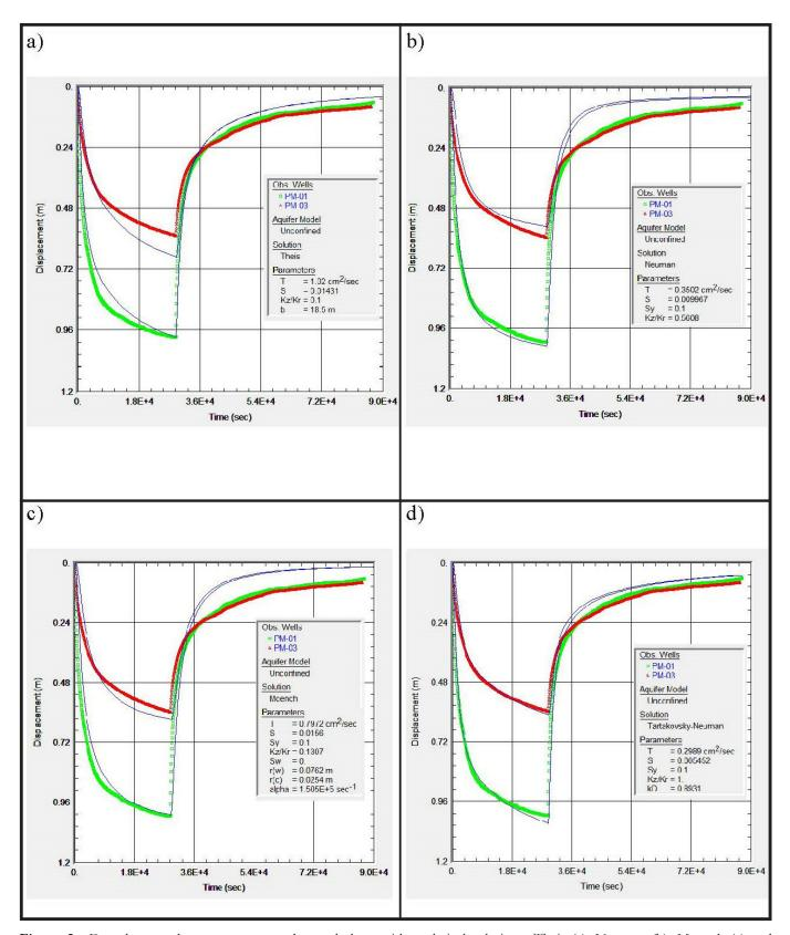
Figure 2. Drawdown and recovery curves observed along with analytical solutions: Theis (a), Neuman (b), Moench (c) and Tartakovsky-Neuman (d).
