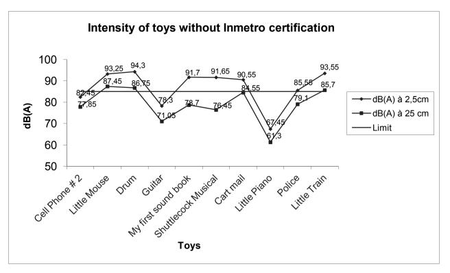
Figure 2 – Average of sound pressure levels (dB) measured from toys without Inmetro certification, at a distance of 2.5 cm and 25 cm (frequency weighting A)
