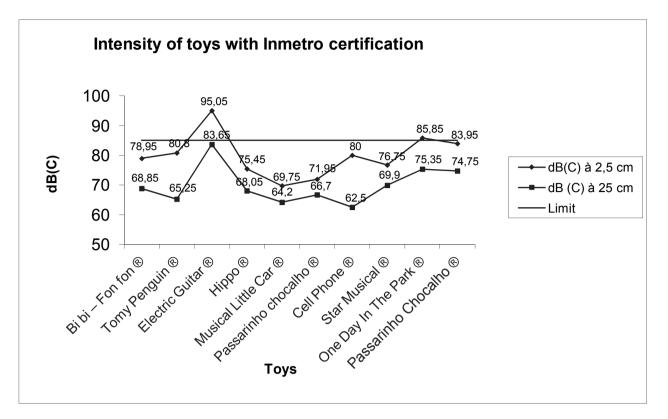
Figure 3 – Average of sound pressure levels (dB) measured from toys with Inmetro certification, at a distance of 2.5 cm and 25 cm (frequency weighting C)
