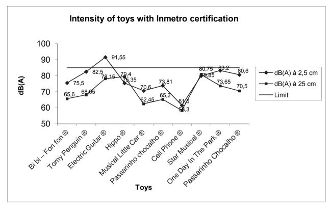
Figure 1 – Average of sound pressure levels (dB) measured from toys with Inmetro certification, at a distance of 2.5 cm and 25 cm (frequency weighting A)
