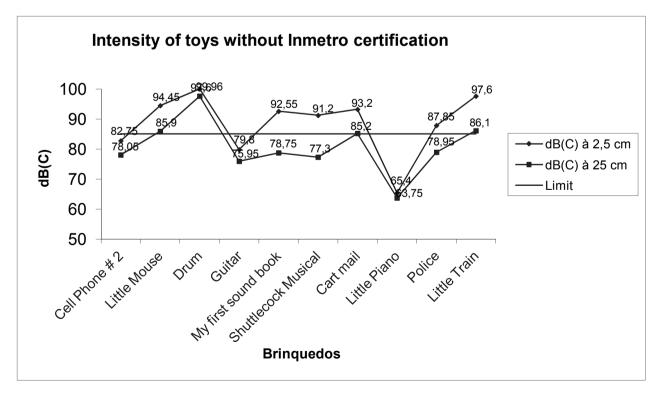
Figure 4 – Average of sound pressure levels (dB) measured from toys without Inmetro certification, at a distance of 2.5 cm and 25 cm (frequency weighting C)
