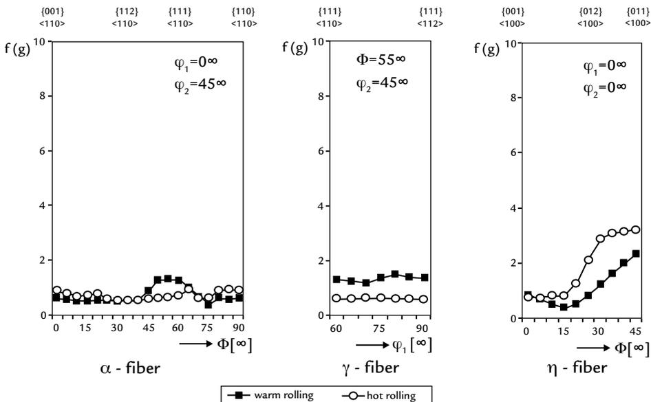
Figure 7 Skeleton lines measured near to the surface ( $s=0.8$ ) of strip.
