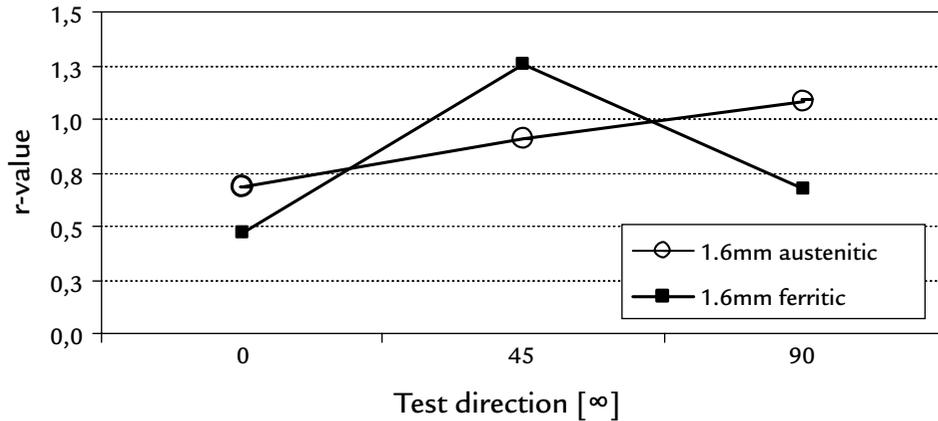
Figure 5 Measured  $r_m$  normal anisotropy values for LC steel ( $t=1.6\text{mm}$ ).
