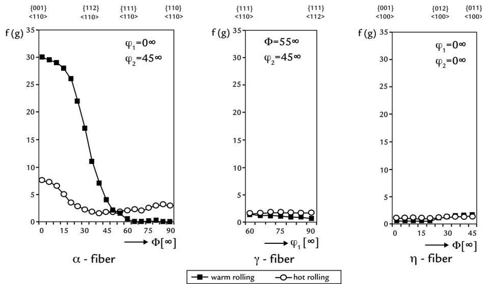
Figure 6 Skeleton lines measured at the center ( $s=0$ ) of strip.
