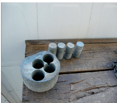
Figure 4 Specimens of 25.54 mm in diameter obtained from original plug 152.4 mm.
