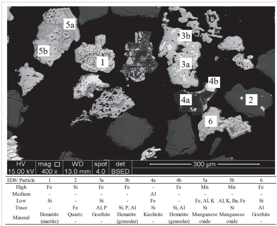
Figure 4 - SEM images for the iron-ore tailings.
