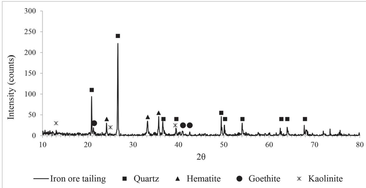
Figure 3 - Tailings mineralogic analysis by XRD – head sample (the background was subtracted).
