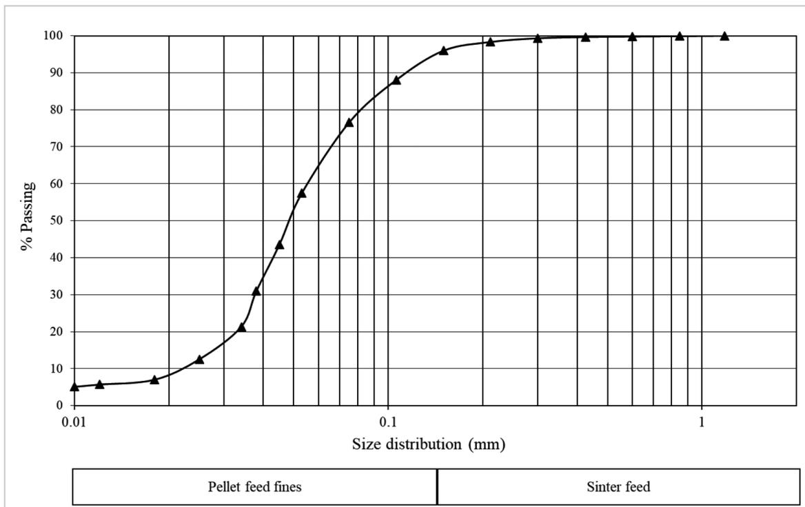
Figure 2 - Iron ore tailings: size distribution.
