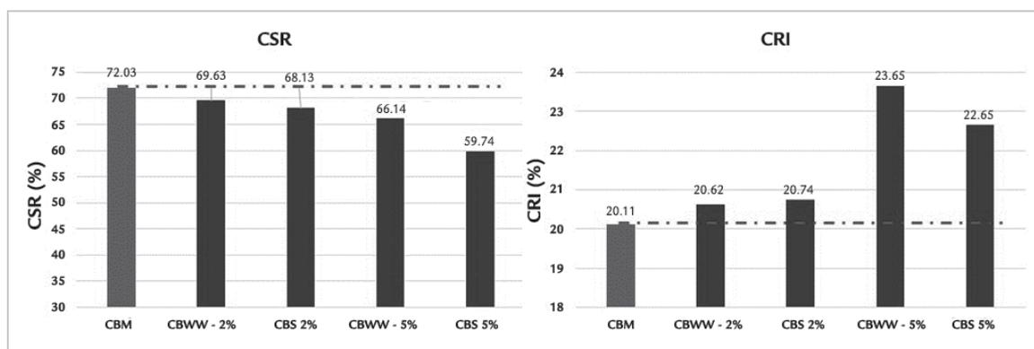
Figure 3 - CSR and CRI of coke produced with different mixtures.
