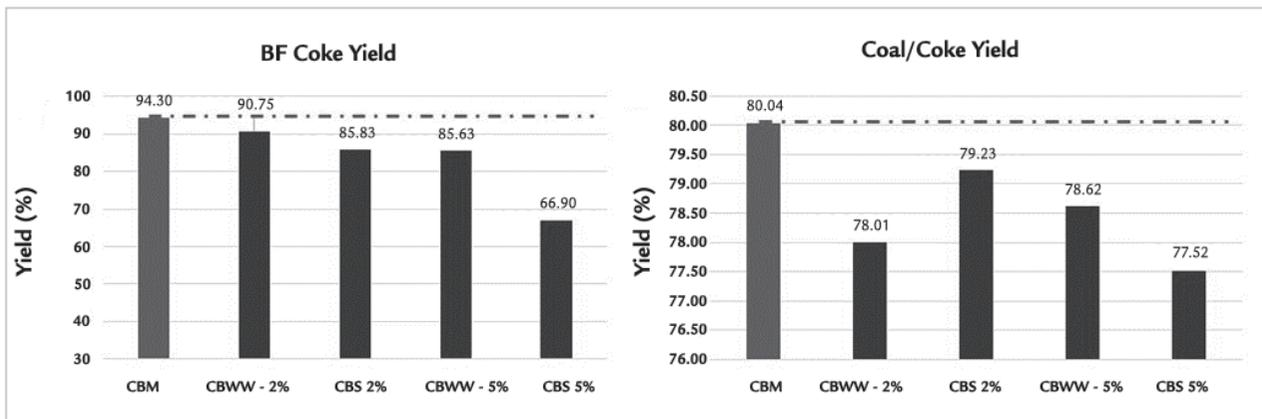
Figure 4 - Results of blast furnace and coke / coal yields.
