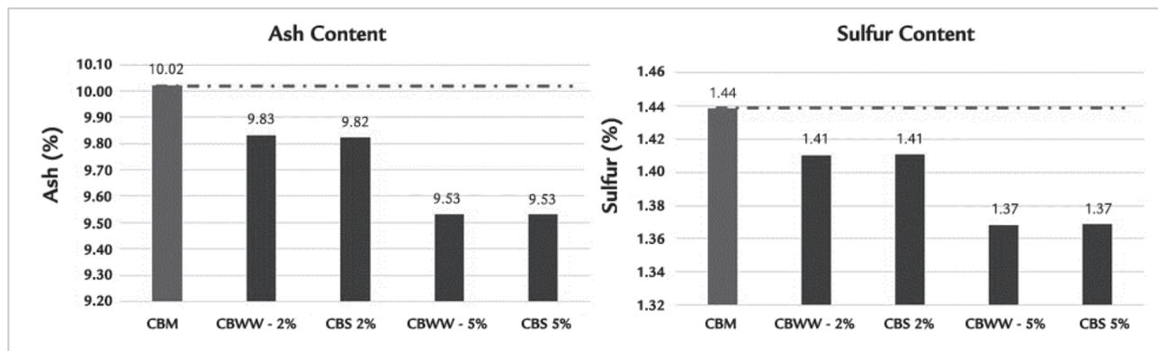
Figure 1 - Ash and sulfur analysis of coke produced with different mixtures.
